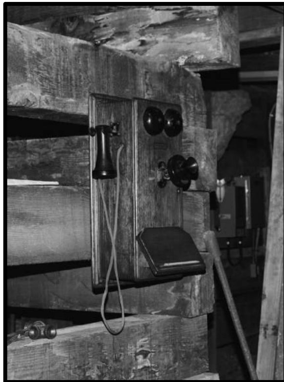
A Western Electric Mine phone originally installed in the Campbell Mine (see p.76, para. 5)
