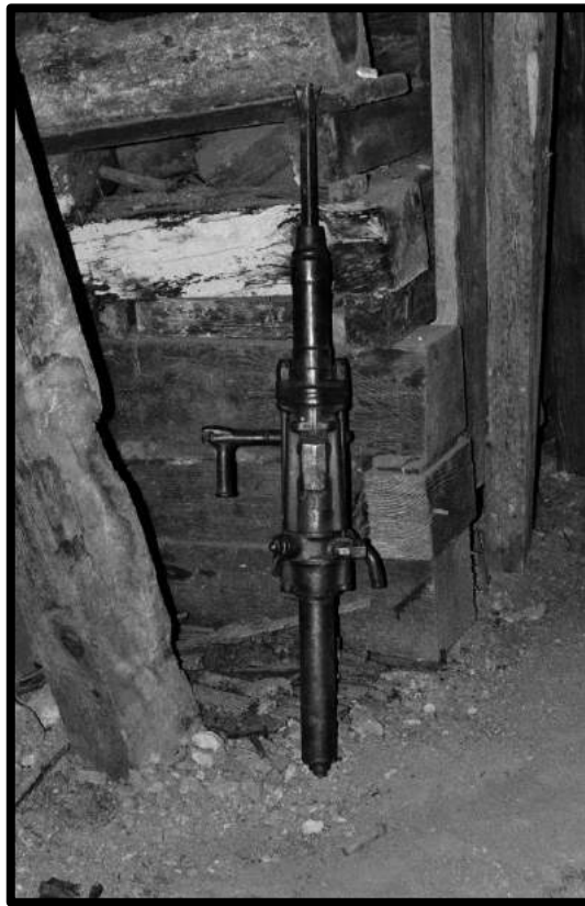
An Ingersoll –Rand stoper with shortened leg (see p73, para. 7)
