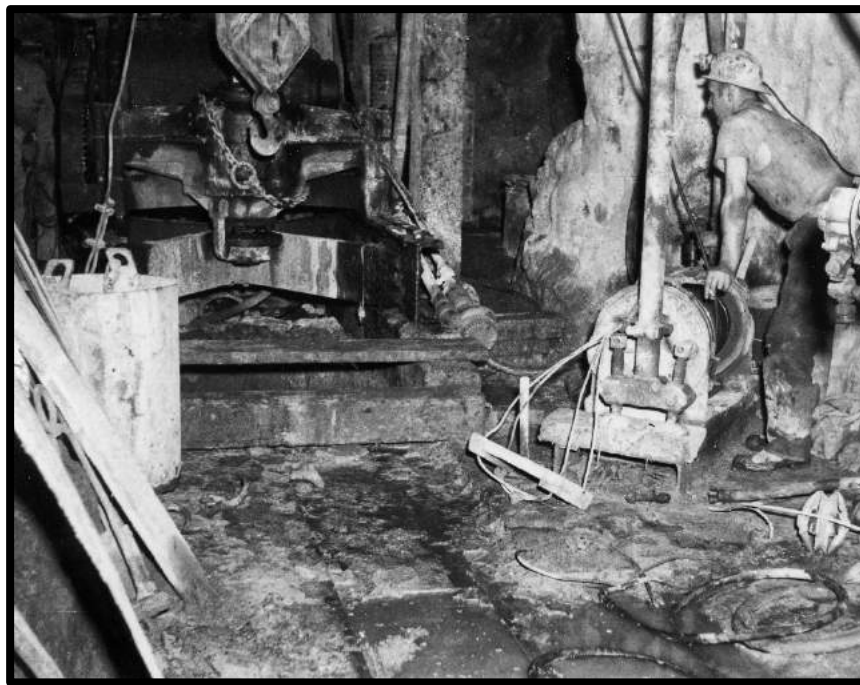
A miner operating a tugging hoist at a Calyx drill (see p.107, para. 2)
