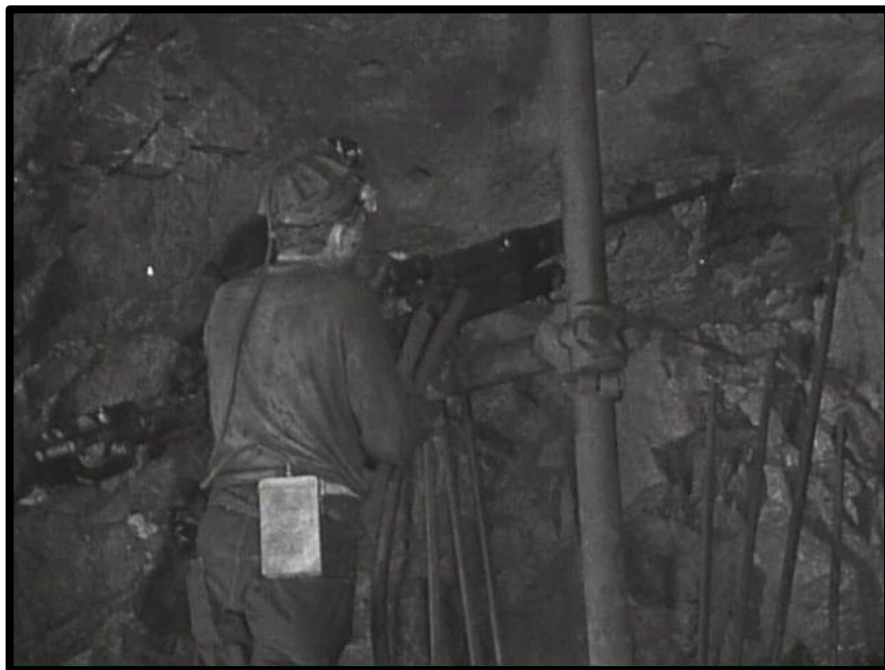
A miner with a model K Edison Lamp drilling in the Campbell Mine. (see p.76, para. 5)
