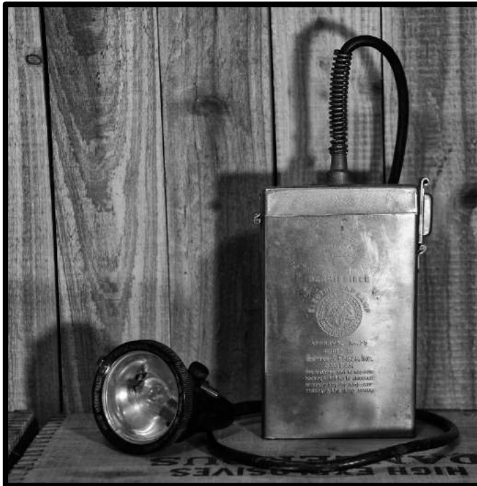
A Model K Edison Cap lamp, the first style used in Bisbee mines (see p.76, para. 5)
