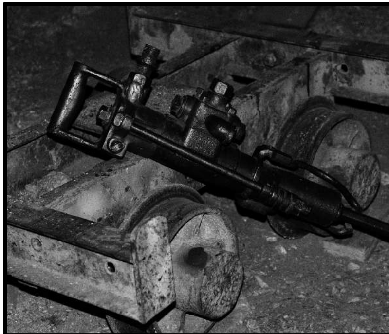
A Cochise brand of plugger drill resting on a timber truck (see p.73, para. 7)
