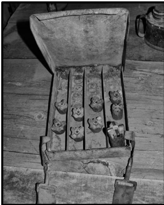
A bit box containing various types of detachable drill bits (see p. 86, para. 4)
