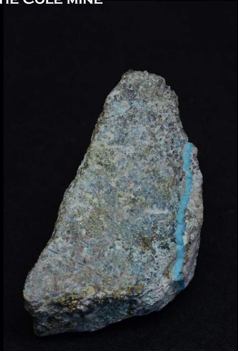
TURQUOISE AS A THIN VEINLET IN A PYRITE/CHALCOPYRITE MIX IN SILICIFIED KAOLINITE, SPECIMEN 4.5 CM.
