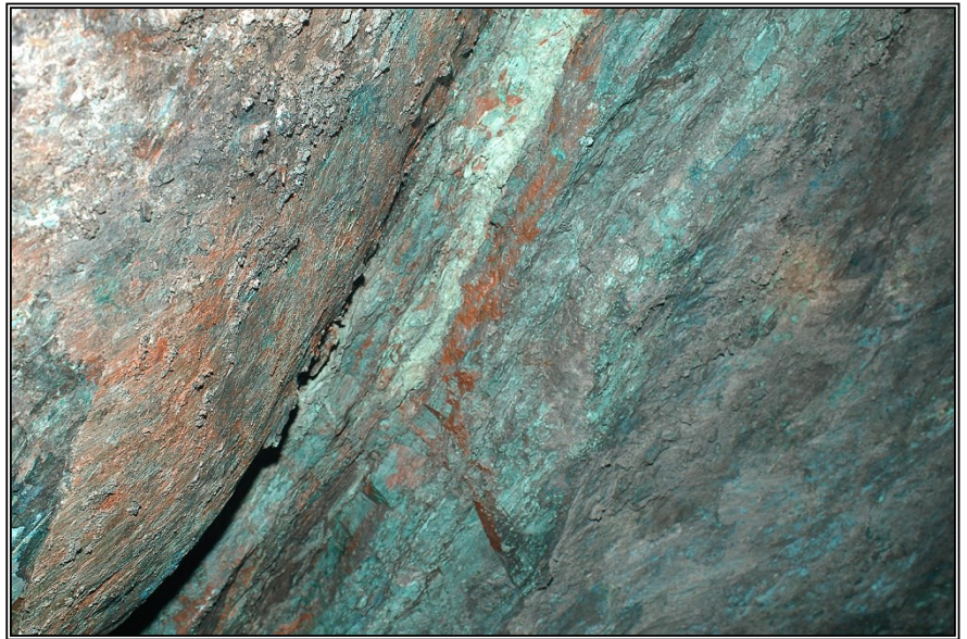
Disseminated supergene chalcocite, as replacements of pyrite in deeply altered limestone, altering to brochantite along a fault. View-1.2 meters, 5 stope, 6 th level Southwest mine. Graeme/Larkin collection.
