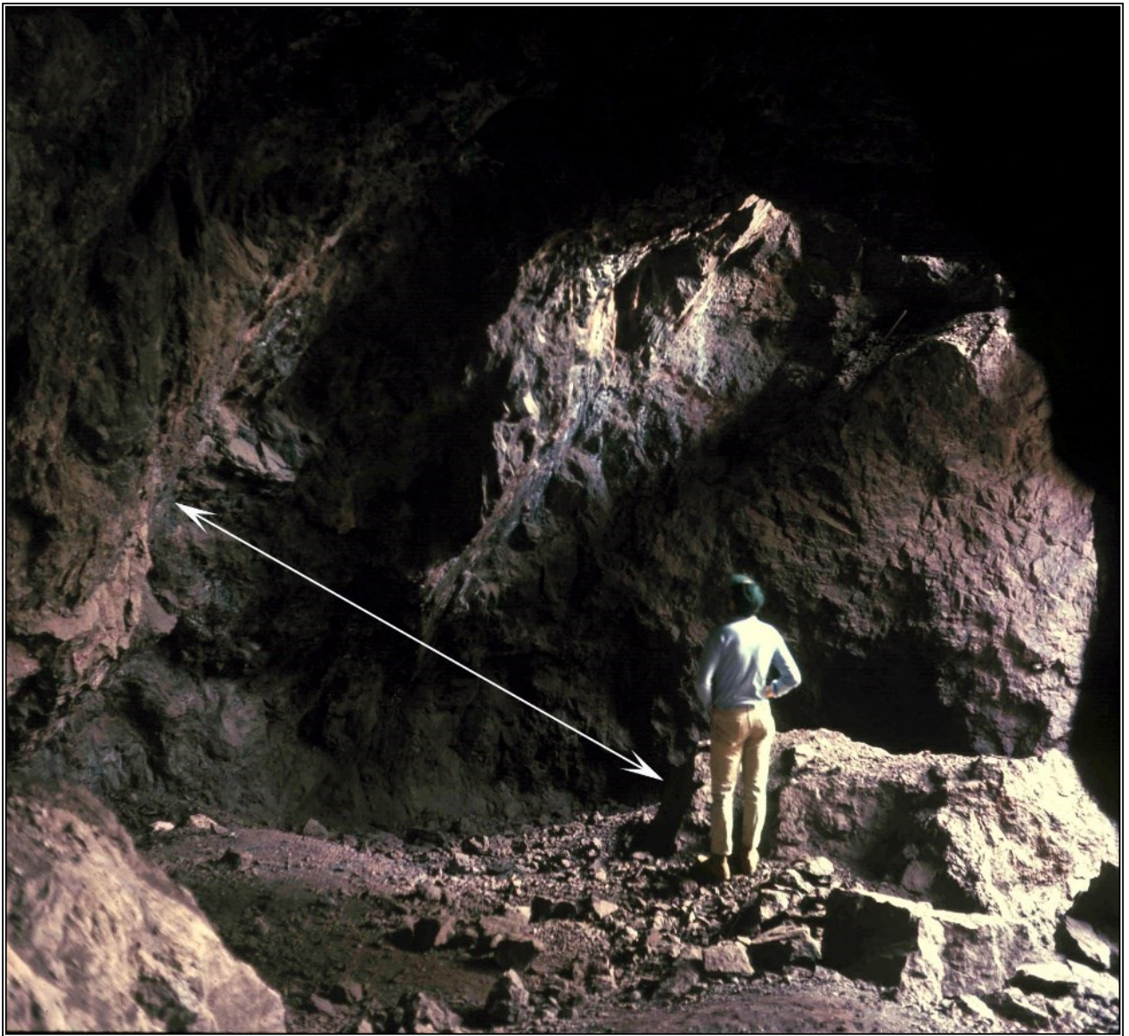
Near-surface manganese stope with the ore zone indicated, Twilight Claim, Higgins Mine – 1967. Graeme/Larkin collection
