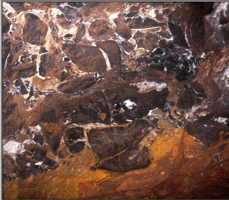
Cross sectional view of breakdown in a cave bottom of altered Martin limestone blocks with some hematite, all cemented by calcite and resting on oxide ores of goethite with malachite. The ore had been mined, leaving only a small amount next to the oxidized breakdown, 100 level, Higgins Mine, horizontal view - 2.7 meters. Graeme/Larkin collection.
