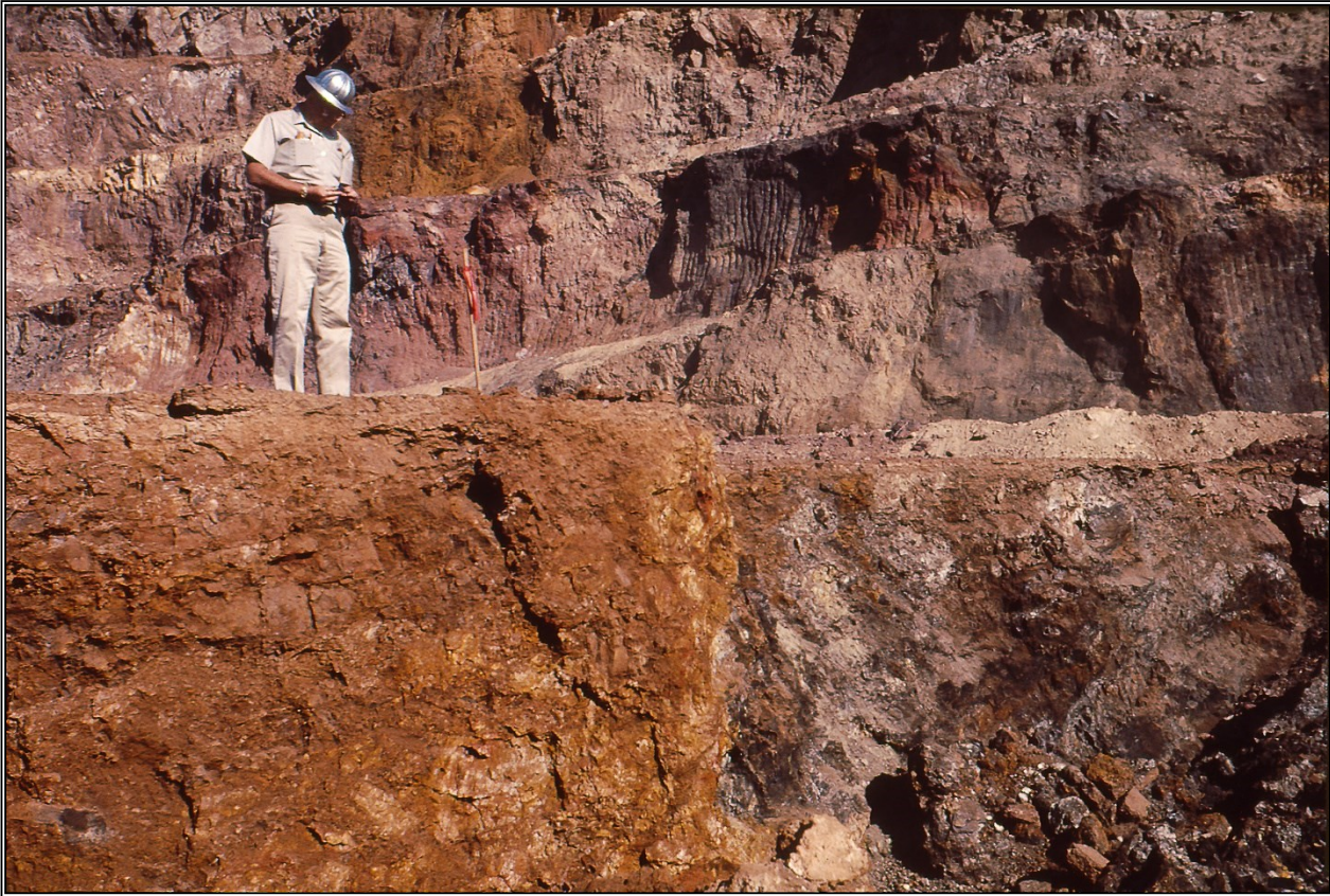
The contact between iron-rich clays and supergene altered limestone in the Holbrook Extension of the Lavender Pit Mine at an elevation of about 5,100 feet. Similar contacts can be seen in several places in the background. The lath with red flagging denotes ore-grade material (>5 percent copper) in the right side. The ore mineral was azurite in this case. A higher copper content was required to make grade as this material was direct shipping ore, as it could not be enhanced by milling, but sent directly to the smelter. The individual in this 1970 photo is Keith Coke, Chief Geologist. Graeme/Larkin collection.
