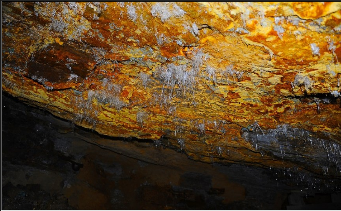
White epsomite, \text{MgSO}_4\cdot 7\text{H}_2\text{O} , efflorescing from Martin limestone, with iron hydroxides as a paint-thick layer on the limestone, 6 th level, Southwest Mine: view – 1.35 meters. Graeme/Larkin collection.
