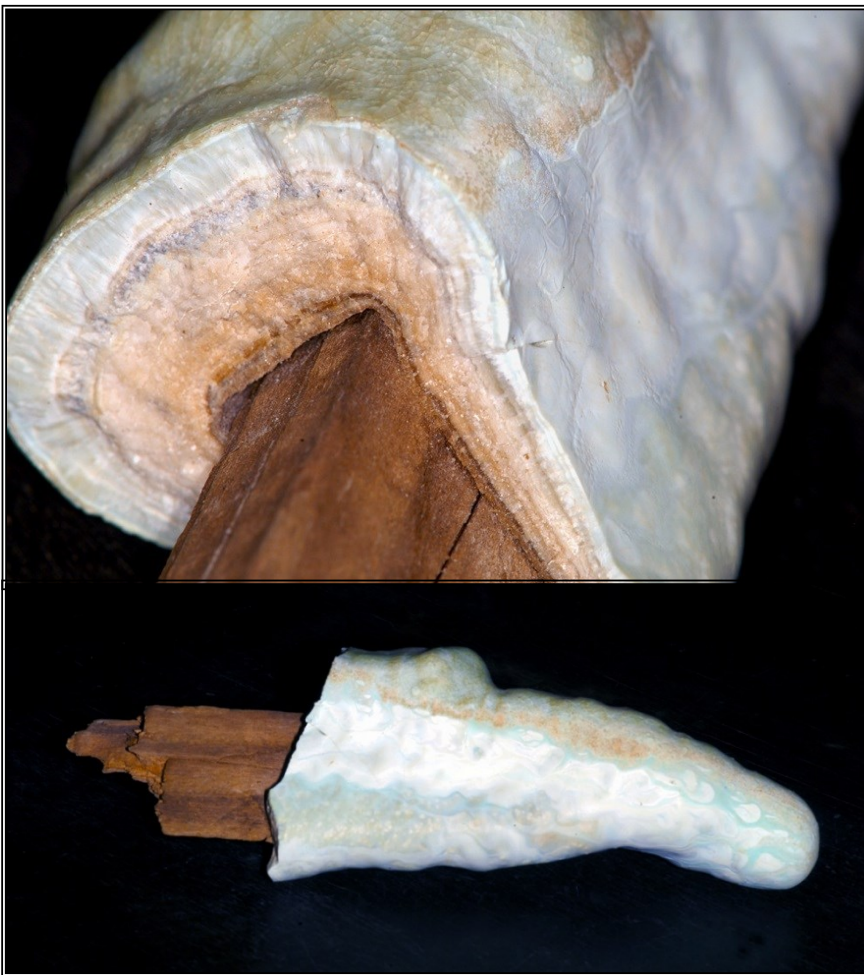
Two views of an 8 cm. aragonite stalactite-like form that grew over broken mine timber in about 25 years. The color variation in the top view, reflects changing water quality from turbid to clear. 2300 level, Junction Mine. Graeme collection.
