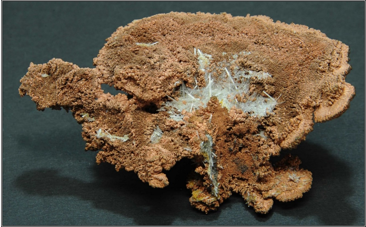
Gypsum, variety selenite, on post-mining copper that precipitated directly from high copper solutions. 2200 level, Junction Mine, specimen – 9 cm. Graeme collection.
