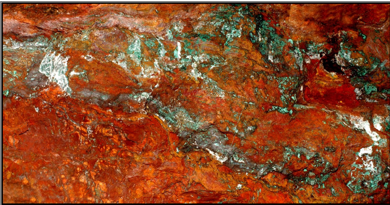
A fully mature, malachite/goethite/hematite supergene orebody with abundant boxwork voids and calcite, which was so common, 5 th level, Southwest Mine, view-2.8 meters, grade \approx 5 percent copper Graeme/Larkin collection.
