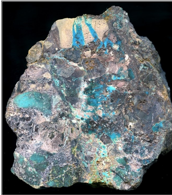
A very complex mix of lithologies composing Glance conglomerate, with turquoise as a filling of minor fractures, replacement of the matrix and as a replacement of clast of varying lithologies. Lavender pit Mine, Specimen-9 cm. Graeme collection.
