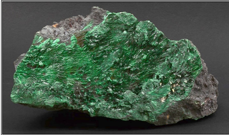
Left: A 22 cm mass of hypogene chalcocite altering to coarsely crystalline malachite. Minor calcite is present. 1500 level, Junction Mine, Graeme collection
