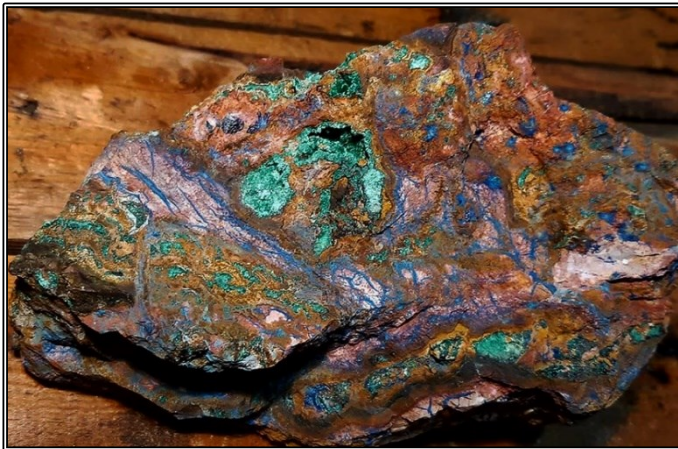
Typical high-grade carbonate ore, > 7% Cu, composed of copper carbonates in a mix of clays/claylike minerals, goethite and altered limestone. 14 stope, 5 th level, Southwest Mine, specimen-20 cm, Graeme collection.
