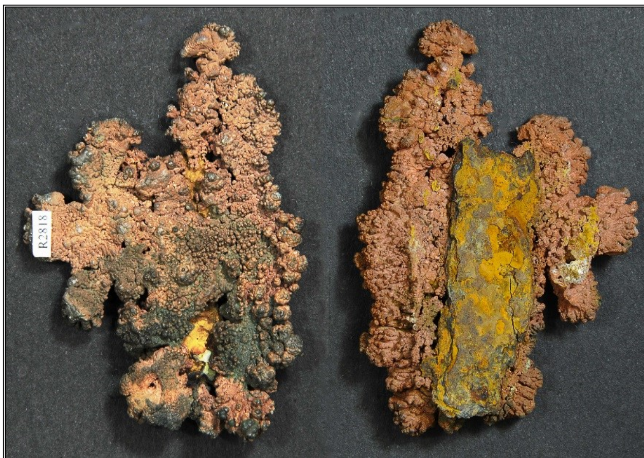
Front and back views of mine rail replaced by copper with the copper expanding well beyond the replaced steel, 2200 level, Campbell Mine, specimen – 10 cm. Graeme collection. The yellow-brown is rust-like material from the iron.
