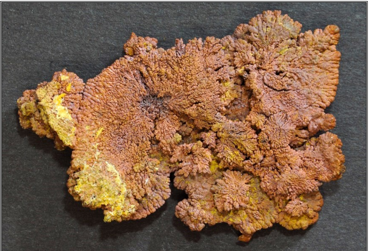
Copper that formed as a direct precipitation from solutions and not replacing steel or iron, 2200 level, Campbell Mine, specimen - 14 cm. Graeme collection.
