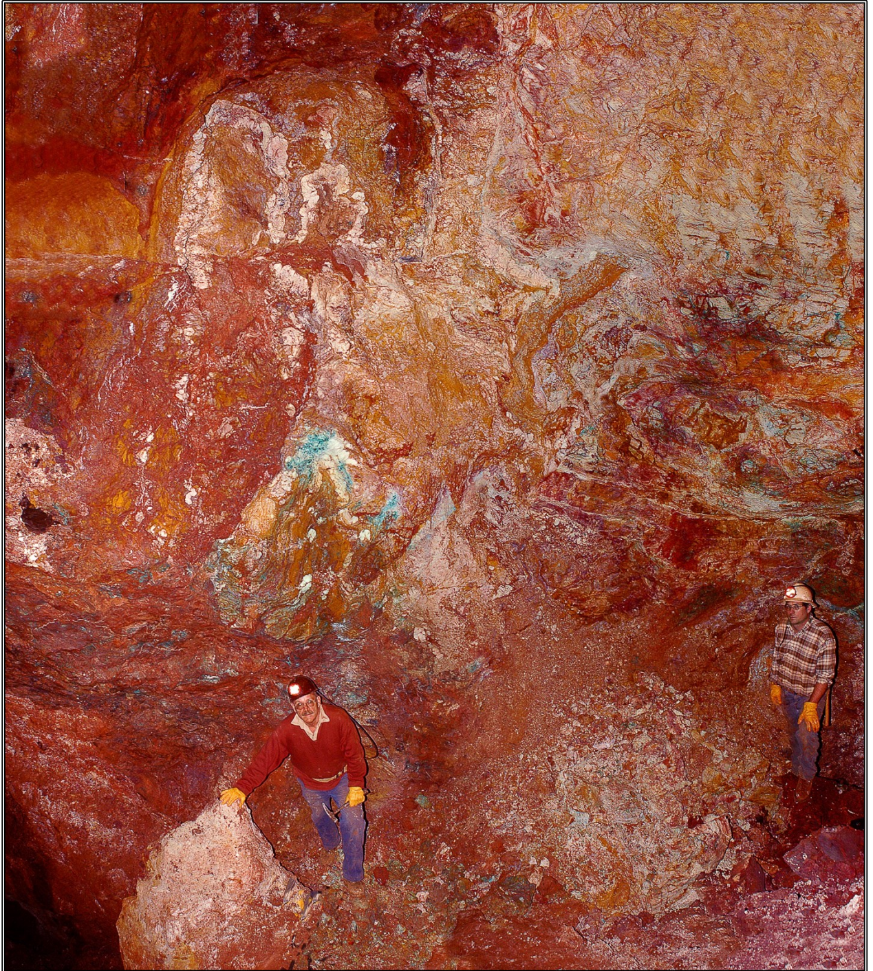
Dr. Peter Williams (left) and author (RWG IV) in front of contorted, supergene clay ores, with cuprite as the principal ore mineral. Areas of cuprite altering to malachite and tenorite are indicated by the green areas. In 12 stope, 6 th and 7 th levels of the Southwest Mine, vertical view-about 10.5 meters. Graeme/Larkin collection.
