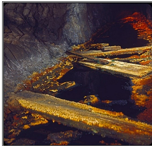
Chalcantite, \text{Cu}^{2+}\text{SO}_4 \cdot 5\text{H}_2\text{O} : (blue) on chalcocite and (green) brochantite, \text{Cu}_4^{2+}(\text{SO}_4)(\text{OH})_6 : on bornite as alteration coatings on broken ore left behind. In situ, 6 th level, Southwest Mine, view – 1.20 meters. Graeme/Larkin collection.
