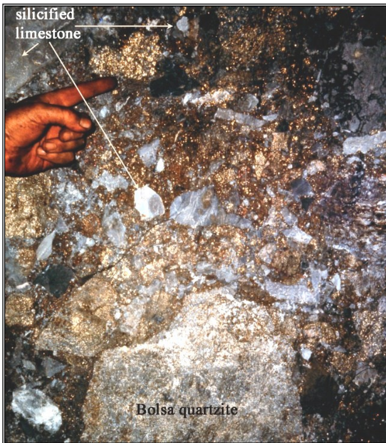
Pyrite replaced fragments, silicified limestone fragments and a large Bolsa quartzite fragment, in intrusive breccia on the 1600 level, Campbell Mine. Graeme/Larkin collection.
