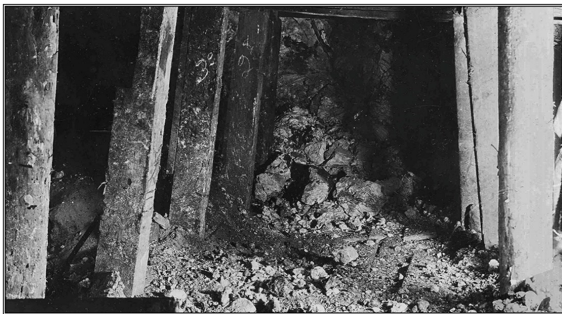
A freshly blasted sulfide muck pile of the intrusion breccia in the Sacramento Mine. The timber to the center-left has numbers written with chalk indicating the copper grade for the material mined behind the post – 3.0% first and then 2.8%; both below ore-grade. The size and number of boulders present tells of hard rock; rock that must be broken by hand to pass through the rock handling system. Photo circa 1918 Graeme-Larkin collection.
