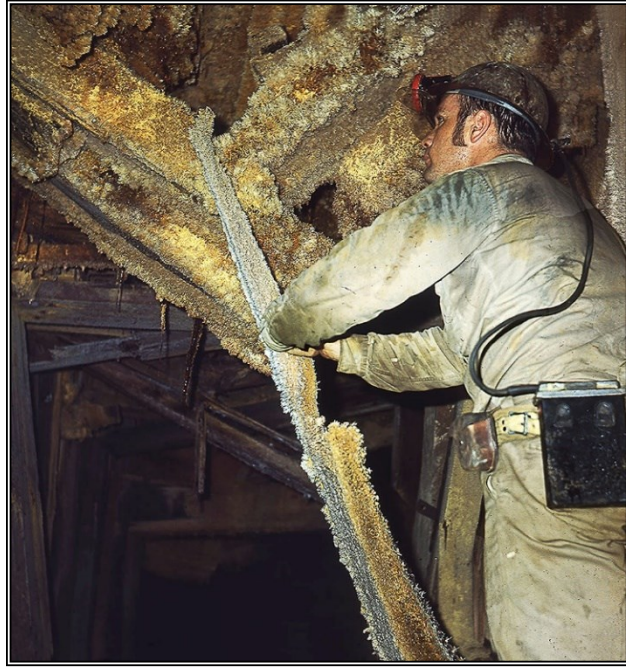
Melanterite, \text{Fe}^{2+}\text{SO}_4\cdot 7\text{H}_2\text{O} , as yellow-brown crystals to 4 cm and still being deposited on broken timbers below a mined-out stope. 2833 level Campbell Mine. Author RWG III is in this 1973 photo. Graeme/Larkin collection.
