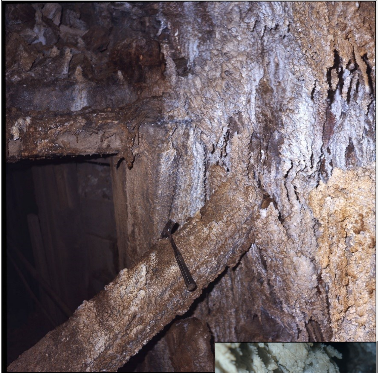
Post-mining calcite deposited by steadily seeping water along a wide fault zone. 2200 level, Junction Mine. Graeme/Larkin collection.
