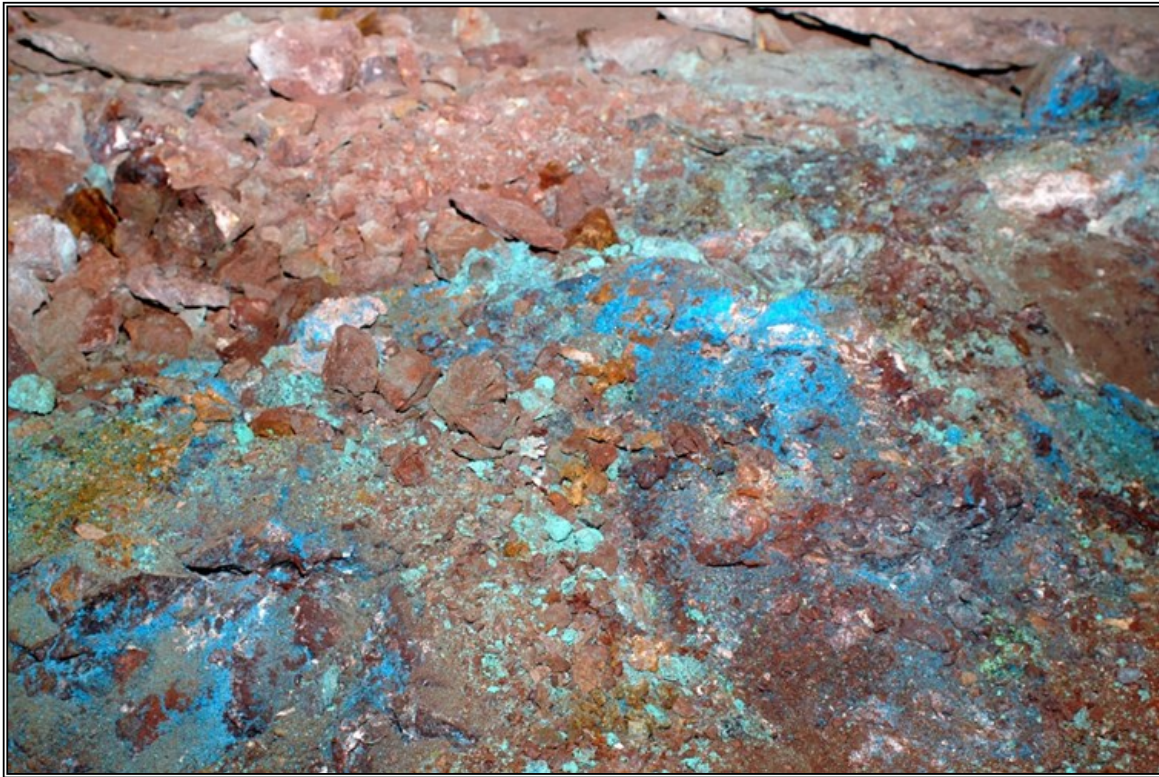
Chalcantite, \text{Cu}^{2+}\text{SO}_4 \cdot 5\text{H}_2\text{O} : (blue) on chalcocite and (green) brochantite, \text{Cu}_4^{2+}(\text{SO}_4)(\text{OH})_6 : on bornite as alteration coatings on broken ore left behind. In situ, 6 th level, Southwest Mine, view – 1.20 meters. Graeme/Larkin collection.
