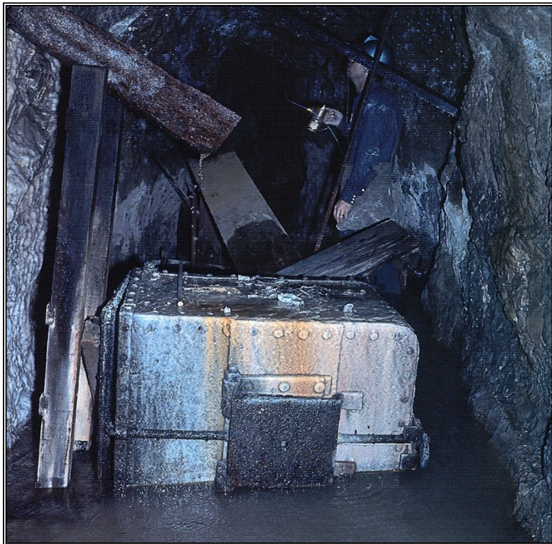
Left top: Post-mining calcite growth on a mine car, Higgins Mine, Tunnel level in 1967. More than 1/2 inch of calcite had been deposited in the just over 20 years since this mine closed.
