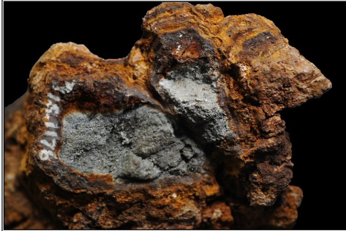
A goethite rind surrounding oxidizing pyrite, specimen-5 cm, Gardner mine, Harvard Museum specimen. Graeme/Larkin collection.
