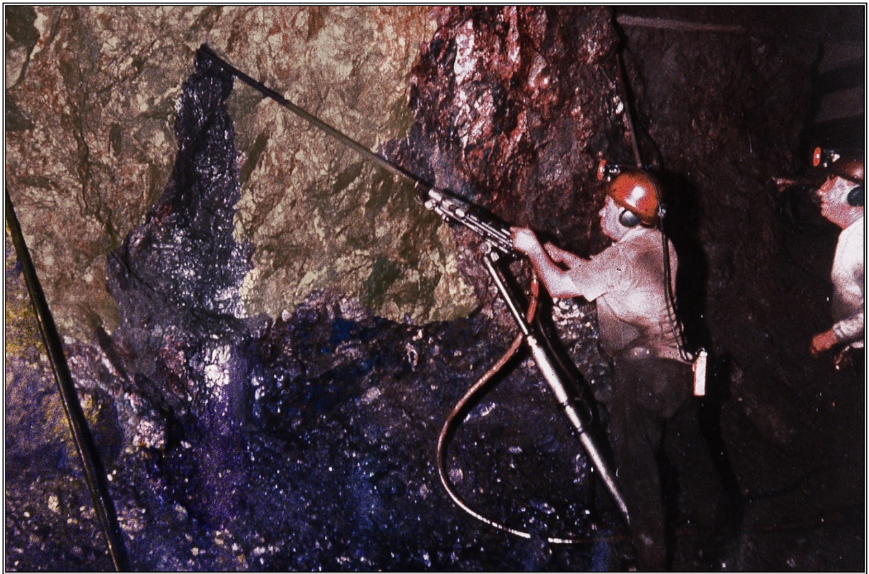
Drilling a blast hole with a jackleg drill in a massive sulfide stope. The minerals are a mix of bornite (lower-1/3), chalcopyrite (left and below of drilling point), pyrite (upper-right corner). The black sludge coming from the drill hole is typical, as all sulfides yield black powder when finely broken. 2833 level, Campbell Mine. The ore from this blast ran 5.8 percent copper. Peter Kresan photo, 1974.
