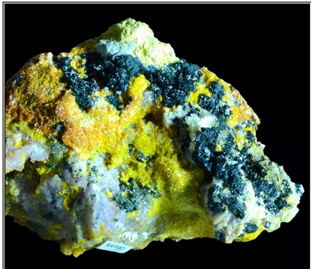
Post-mining crust of coquimbite, \text{Fe}_2^{3+}(\text{SO}_4)_3 \cdot 9\text{H}_2\text{O} : (light purple), paracoquimbite, \text{Fe}_2^{3+}(\text{SO}_4)_3 \cdot 9\text{H}_2\text{O} : (light purple), copiapite, \text{Fe}^{2+}\text{Fe}^{3+}(\text{SO}_4)_6(\text{OH})_2 \cdot 20\text{H}_2\text{O} : (yellow), melanterite \text{Fe}^{2+}\text{SO}_4 \cdot 7\text{H}_2\text{O} : (white), voltaite, \text{K}_2\text{Fe}_5^{2+}\text{Fe}_4^{3+}(\text{SO}_4)_{12} \cdot 18\text{H}_2\text{O} : (black). Lavender Pit Mine, view - 8 cm. Graeme collection.
