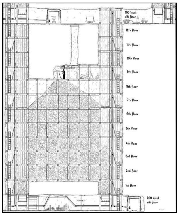
Diagram showing the floors between levels for an area where the levels are 100 feet apart. Sill level is 10 feet high, while the other floors are 8 ½ feet high.
