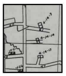
Series of raises with three number names. These raises were driven from the 4<sup>th</sup> level of the Southwest Mine and Intercepted 5<sup>th</sup> level workings (Note, in the Southwest Mine the 5<sup>th</sup> level is above the fourth level.
