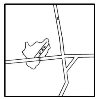
1'' = 50' scale map with the stope drawn as a solid line, Note that 6-64 and part of 9 crosscuts have been mined out
