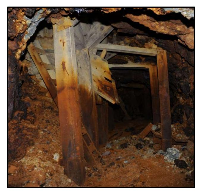
Double compartment raise, one chute compartment and one manway. 6<sup>th</sup> level Southwest mine.
