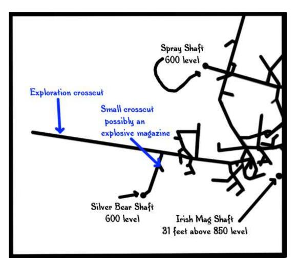
Long crosscuts driven were driven in exploration of ore. To a mineral collector these are of less interest since they normally were in waste rock and are less likely to contain interesting minerals. Short prospecting crosscuts are of more interest. These workings were often converted into tool rooms, explosive magazines and timber stations. As a result they may contain interesting mining relics.
