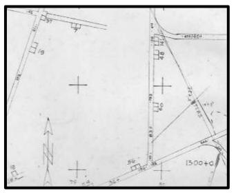
The Calumet & Arizona simply numbered the raises in the order they were driven on the level.
