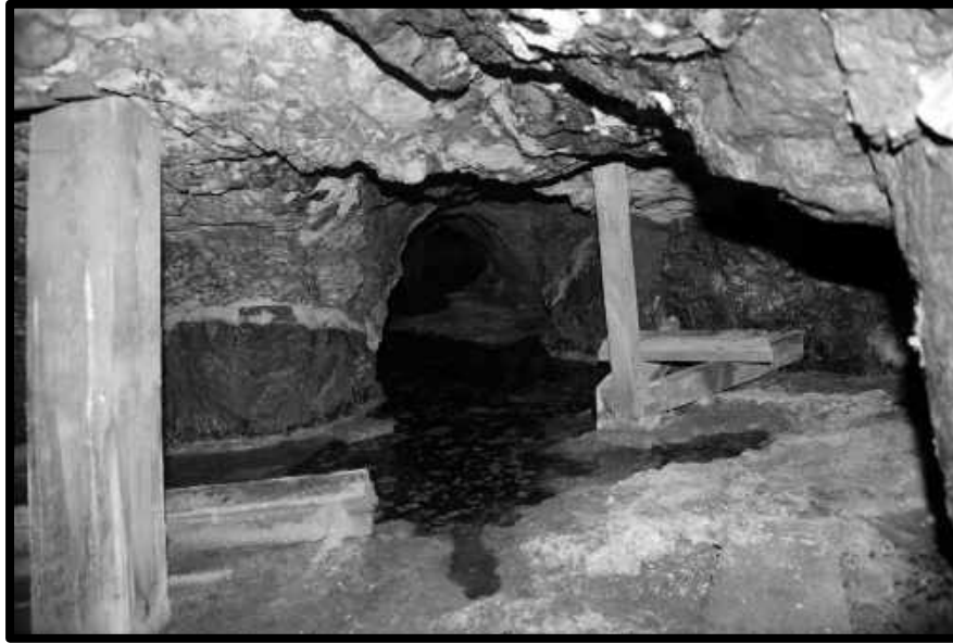
An abandoned drift flooded with “copper water” on the 6 th level Southwest mine.
