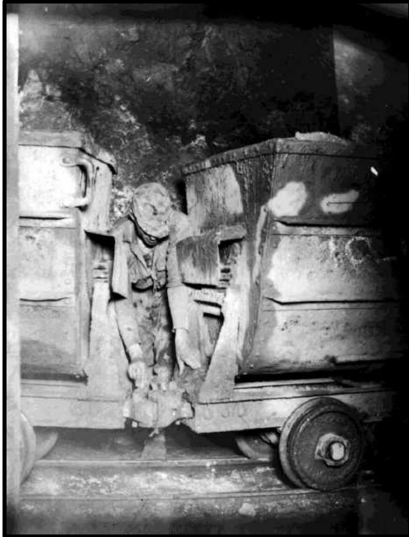
A safety photo showing a miner unsafely coupling two mine cars, c-1917
