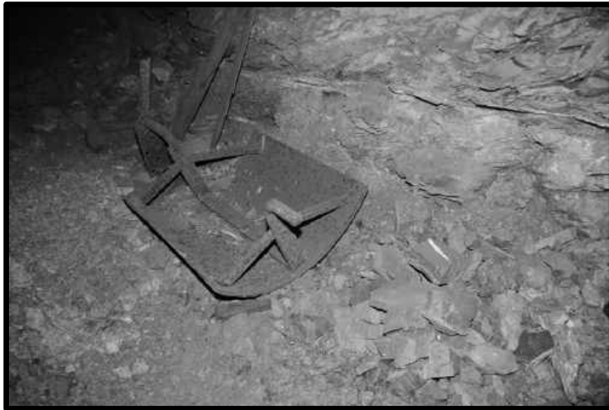
A chute door laying at the side of a crosscut, 3 rd level Southwest Mine.
