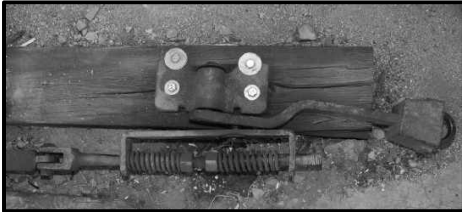
Two different types of switch throws, above and below
