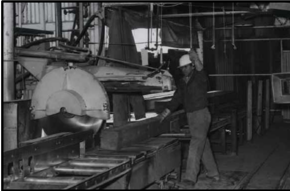
Cutting 8”X 8” timber in the Junction Mine Saw Mill c-1960
