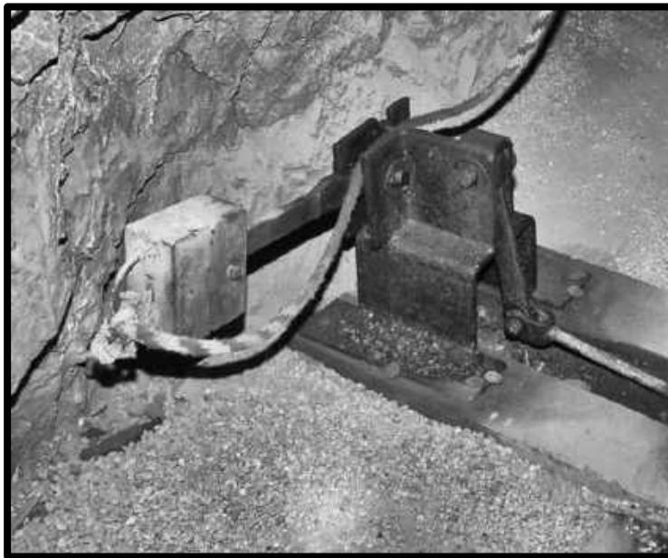
Two different types of switch throws, above and below
