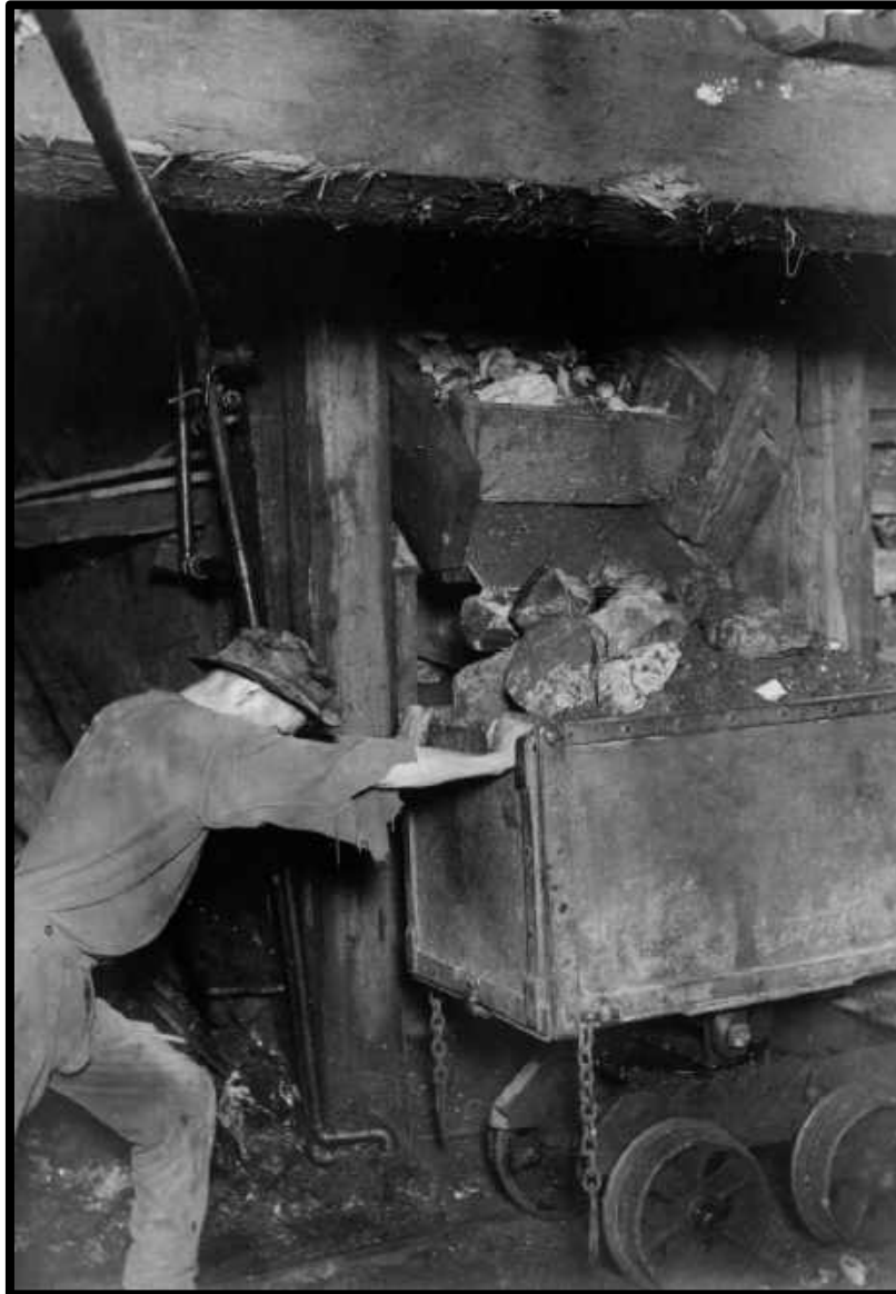
Safety photo showing a miner risking his fingers by placing them over the edge of a mine car tub. C-1917
