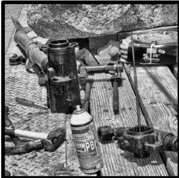
A Gardner-Denver Model 63 jack leg drill being repaired at the Queen Mine
