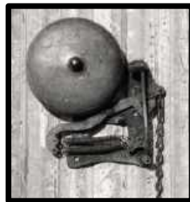
Mechanical call bell from the Czar hoist house
