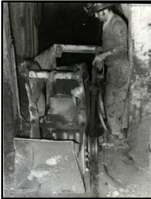
A miner in Bisbee operating a mucking machine. Notice, the narrow working conditions.
