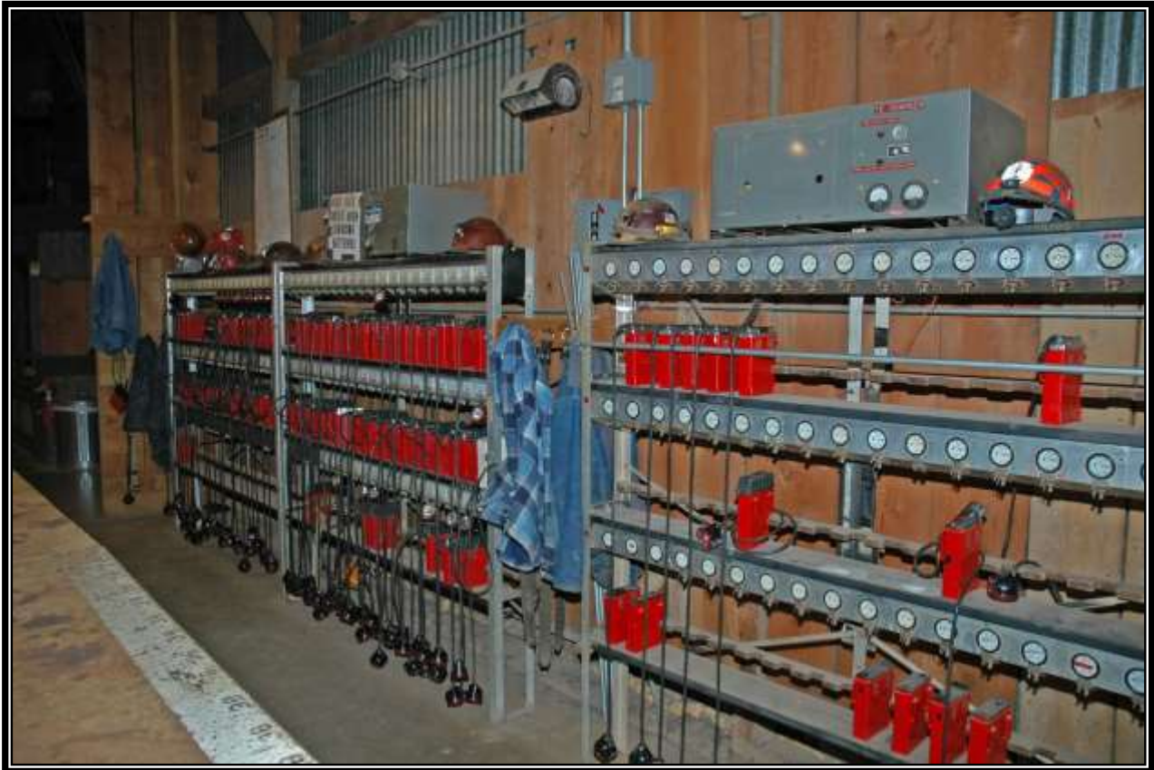
Lamp charging rack at the Queen Mine Tours was identical to those used in the mines from 1967 to 1975 Graeme Larkin collection
