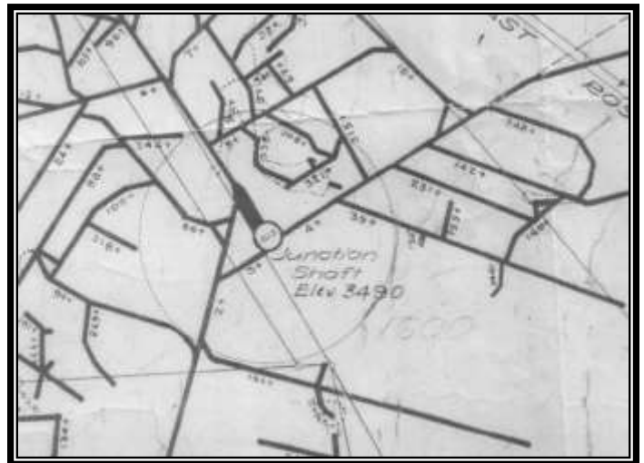
A map of a part of the 1600 level of the Junction Mine with the 200' diameter shaft pillar clearly marked as a circle. C-1950
