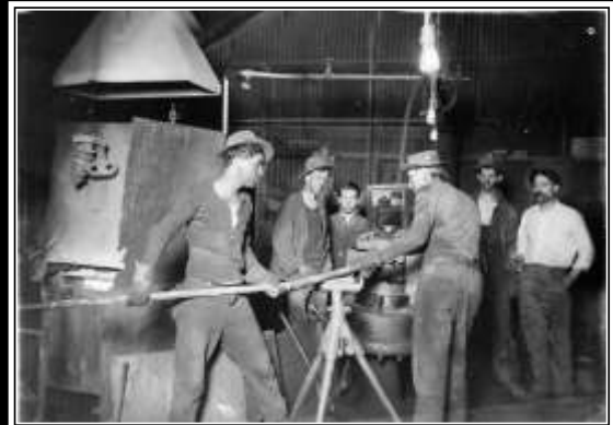
GRAEME LARKIN COLLECTION SHARPENING DRILL STEEL IN THE CQ BLACKSMITH SHOP C- 1916
