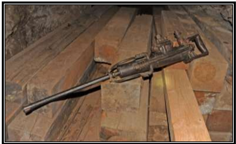
Cochise brand plugger drill ad (top) and an example below, both C - 1920 Graeme Larkin collection
