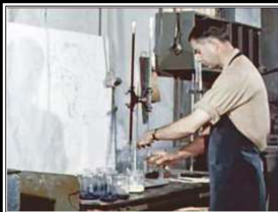
GRAEME LARKIN COLLECTION A WET DETERMINATION FOR COPPER CONTENT IN THE ASSAY OFFICE AT BISBEE - 1950
