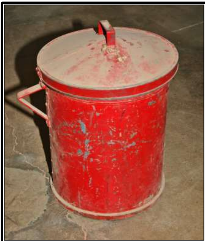
LEFT – FUSE CAN OF THE TYPE USED TO TRANSPORT FIRE FUSE ALREADY CUT TO LENGTH WITH THE BLASTING CAPS ATTACHED FROM THE FUSE HOUSE AT THE JUNCTION MINE TO THE VARIOUS POWDER MAGAZINES QUEEN MINE TOURS COLLECTION
