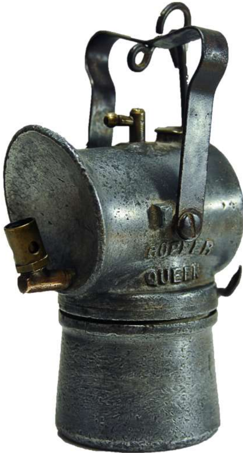
Justrite aluminum stope lamp model 110, as made specifically for the Copper Queen Consolidated Mining Company C- 1915.
