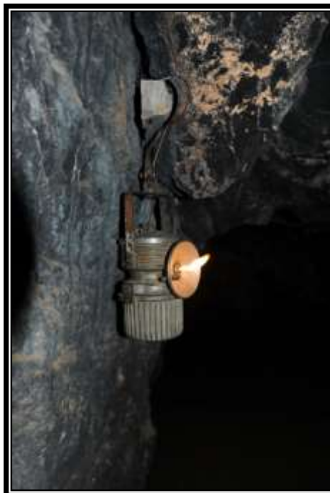
Left: A stope type carbide lamp in use. Graeme Larkin collection
