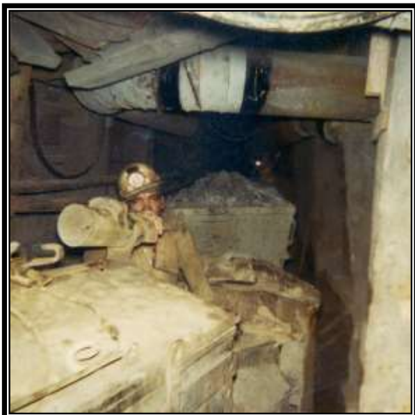
Several styles of storage battery locomotives were used successfully in the mines as well. The small “Mancha” trammers was common, while the eight ton locomotive, such as that show at the left were less common.
