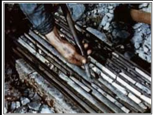
GRAEME LARKIN COLLECTION DIAMOND DRILLING CORE BEING REMOVED FROM CORE BARREL CAMPBELL MINE -1950
