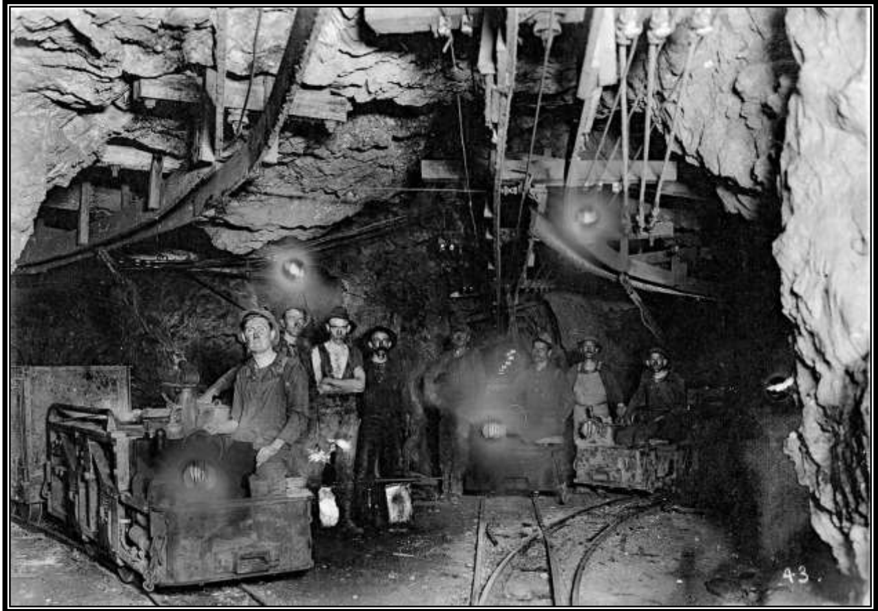
Three trolley motors of varying size on the 1600 level of the Junction Mine, C – 1916. This was a main haulage level where ores from the Briggs and Hoatson mines as well as the Junction stopes on this level were all collected and brought to the Junction Shaft for hoisting.
