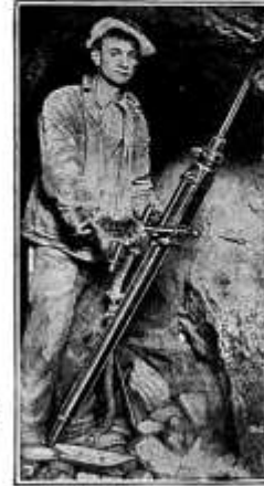
One of 60 “Waugh” Stopers in the Boulder Tungsten Mine.
