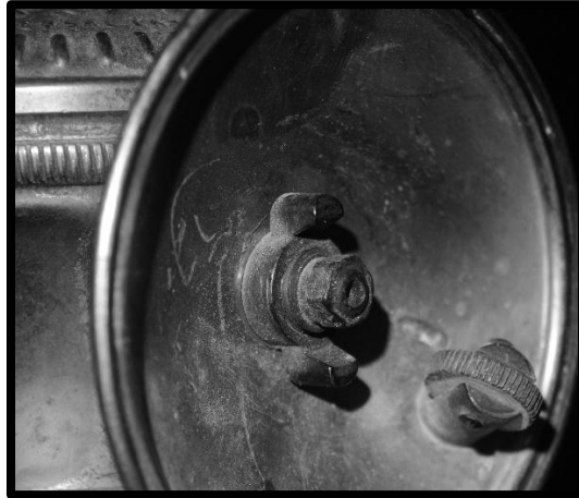
DIAMOND TIP , IN A WELL-USED IN AN AUTOLITE CARBIDE CAP LAMP
