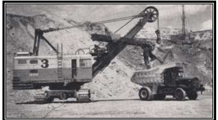
A P&H model 1600 electric shovel loading a 25-ton capacity Mack haul truck in the Lavender PIT Mine – 1953. Graeme Larkin collection
