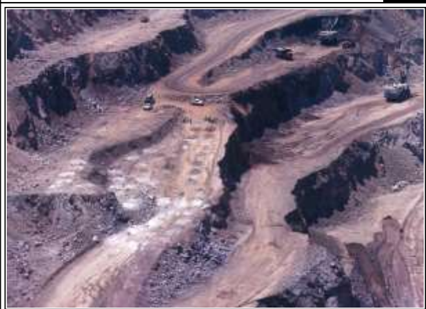
POWDER CREW LOADING BLAST HOLES, 1970. NOTE THE DIFFERENCE IN COLORS IN THE BLAST HOLE CUTTINGS GRAEME LARKIN COLLECTION
