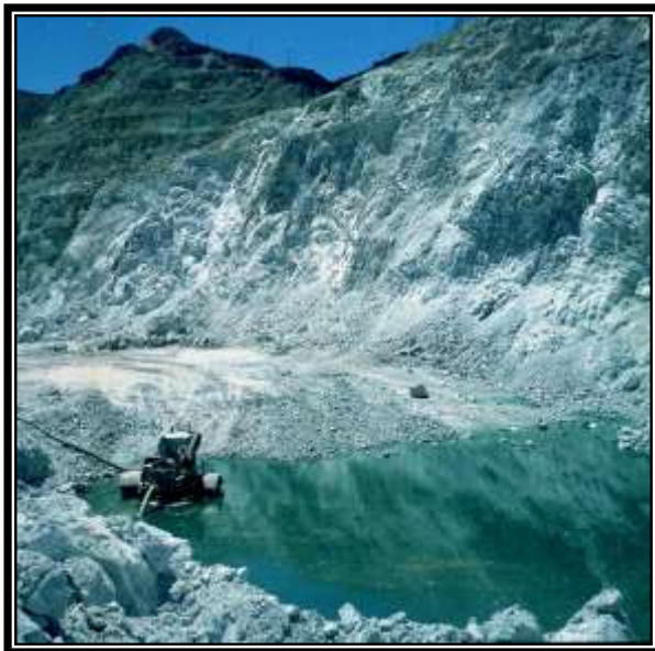
Above: Ponded, high copper content – low pH water being pumped out of a drop cut following a summer rain – 1962. Right: Mine timber from a raise intersected during mining in the pit – 1970.
