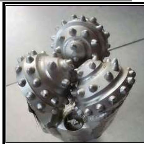
A Timken tri-cone drill bit similar to those used at Bisbee
