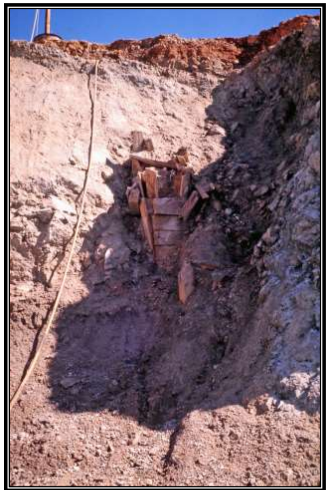
Above: Ponded, high copper content – low pH water being pumped out of a drop cut following a summer rain – 1962. Right: Mine timber from a raise intersected during mining in the pit – 1970.
