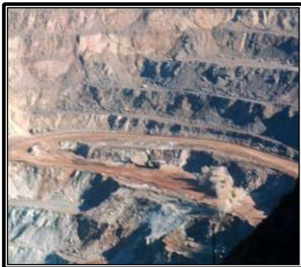
A bank or primary blast on the east wall of the pit – 1966. The amount of heave (displacement) by the blast can be judged by the photo above. The close proximity of equipment to the blast is proof enough that little rock was thrown any distance Graeme Larkin collection
