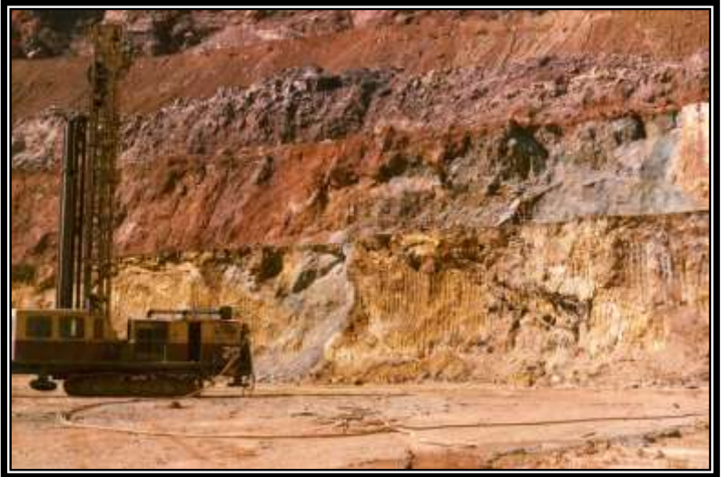
Bucyrus Erie 50 R rotary drill in the Holbrook Extension of the Lavender Pit – 1970. This drill was capable of drilling 12" diameter holes to a depth of 55 feet. These drills operated on 2300 volts that was delivered the heavy insulated cable in the foreground.
