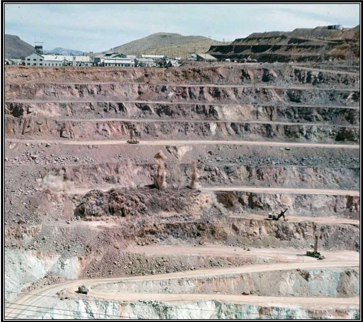
A bank or primary blast on the east wall of the pit – 1966. The amount of heave (displacement) by the blast can be judged by the photo above. The close proximity of equipment to the blast is proof enough that little rock was thrown any distance Graeme Larkin collection
