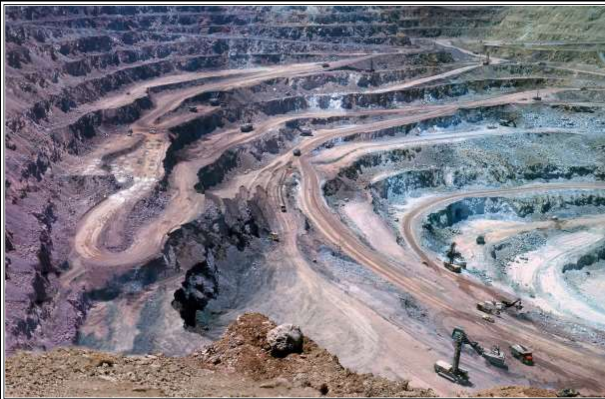
CUTBACK ON THE SOUTH WALL — 1966. THE WIDE SPACES REPRESENT THE REMOVAL OF THE RED/BROWN OVERBURDEN FROM THE GRAY ORE TO MAKE IT AVAILABLE. A FULL SEVEN SHOVELS CAN BE SEEN IN THIS VIEW, FOUR MINING ORE AND THREE IN OVERBURDEN, REFLECTING THE ADVANCED STAGE OF THIS CUTBACK.
