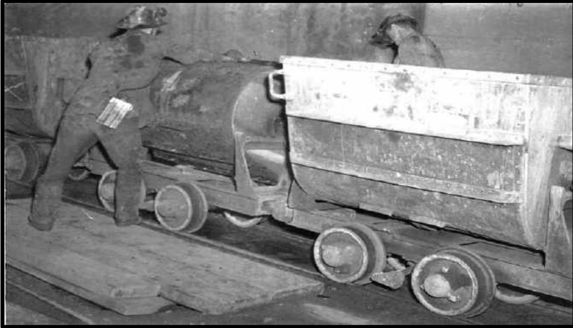
ROCKER DUMP (E-CARS) BEING DUMPED IN AN UNDETERMINED MINE AT BISBEE.
