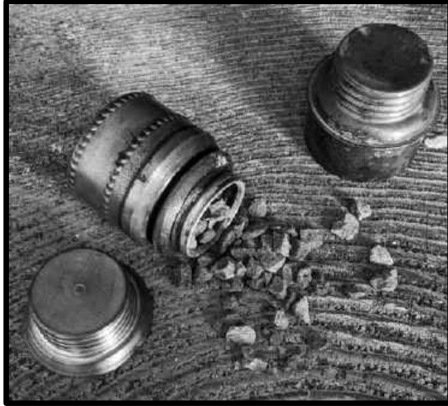
CARBIDE SPILLING FROM A SPARE CARBIDE LAMP BOTTOM
