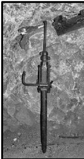
WIDOW MAKER , "WAUGH" STOPER MADE BY DENVER ROCK DRILL SOUTHWEST MINE, 3 RD LEVEL, 30 CROSSCUT.
