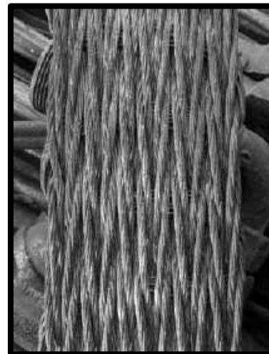
FLAT ROPE (ABOVE) CLOSE UP VIEW RECOVERED FROM 3 RD LEVEL SOUTHWEST MINE
