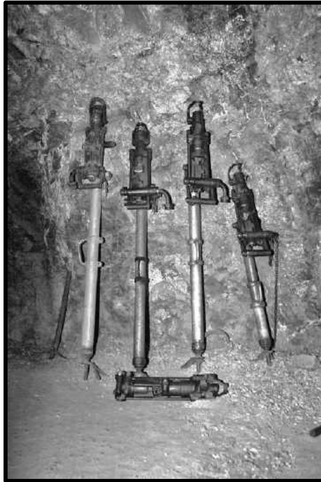
JACKLEG (S) ABOVE ARE THE MODELS USED IN BISBEE DURING ACTIVE MINING. LEFT TO RIGHT THOR 300, GARDNER-DENVER S58F, GARDNER DENVER S63F, GARDNER-DENVER S63F ON A SHORT LEG AND ON THE GROUND WITHOUT A LEG IS AN INGERSOLL-RAND JR 38
