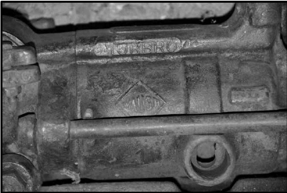
TURBO DRILL , CLOSE UP OF THE VALVE CHEST.
