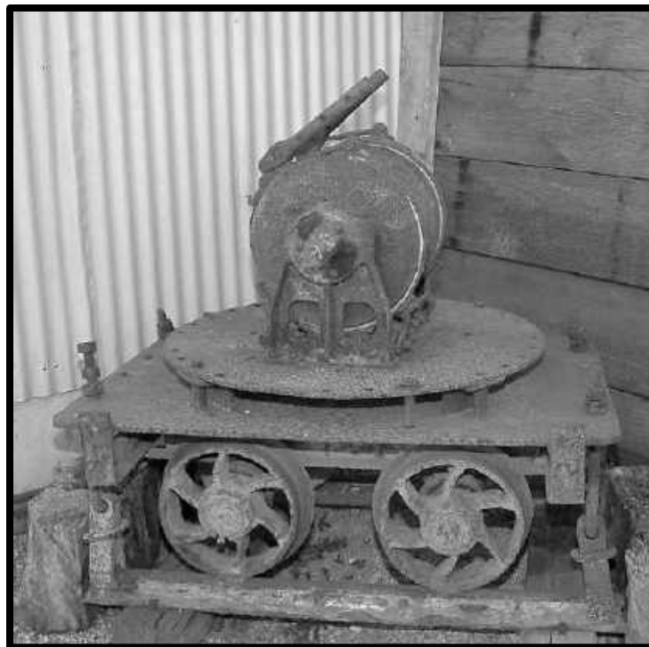
TUGGER MOUNTED ON A SET OF TRUCKS AT THE QUEEN MINE TOUR.
