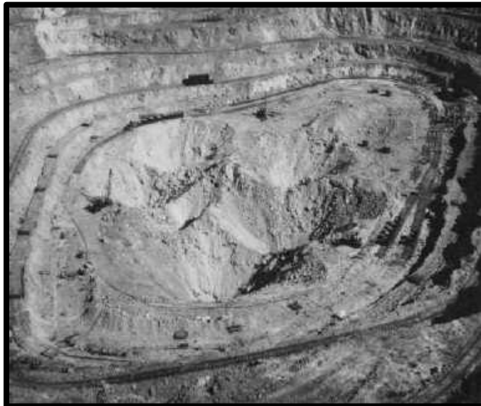
GLORY HOLE (DEF. 1) GLORYHOLES IN THE BOTTOM OF THE SACRAMENTO PIT. THREE CHURN DRILLS ARE DRILLING BLAST HOLE PATTERNS ON THE EDGES OF THE GLORYHOLES TO BE LATER BLASTED INTO THE HOLES.
