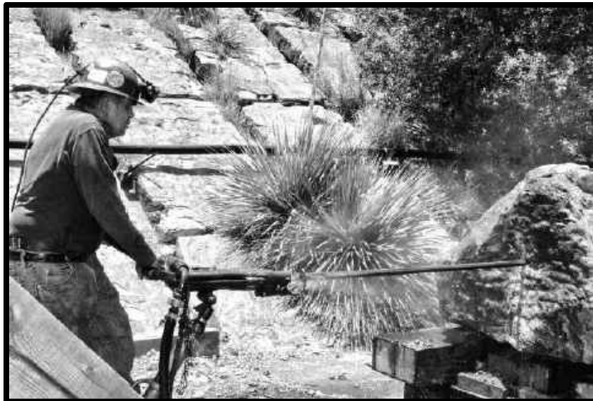
COLLARING A MINER COLLARING A HOLE TO TEST A REPAIRED A GARDNER DENVER S63F JACKLEG.
