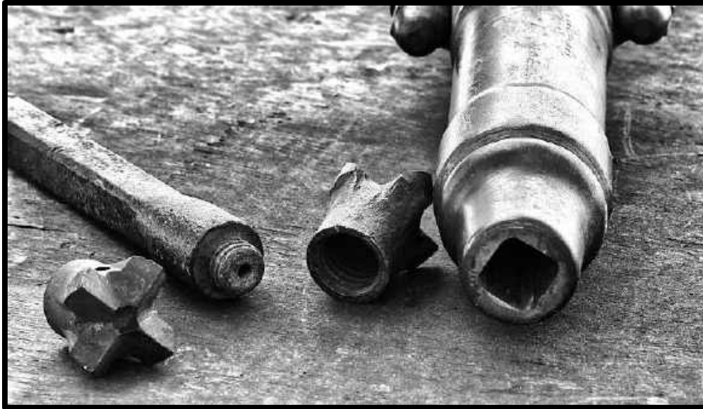
SCREW-OFF BIT(S) WITH A DRILL STEEL AND AN INGERSOLL-RAND 45 STOPER
