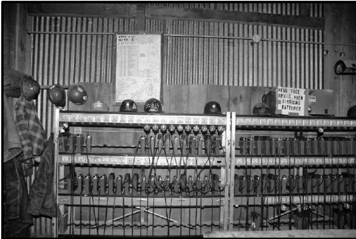
LAMP RACKS WITH WHEAT MARK V LAMPS AT THE QUEEN MINE TOUR
