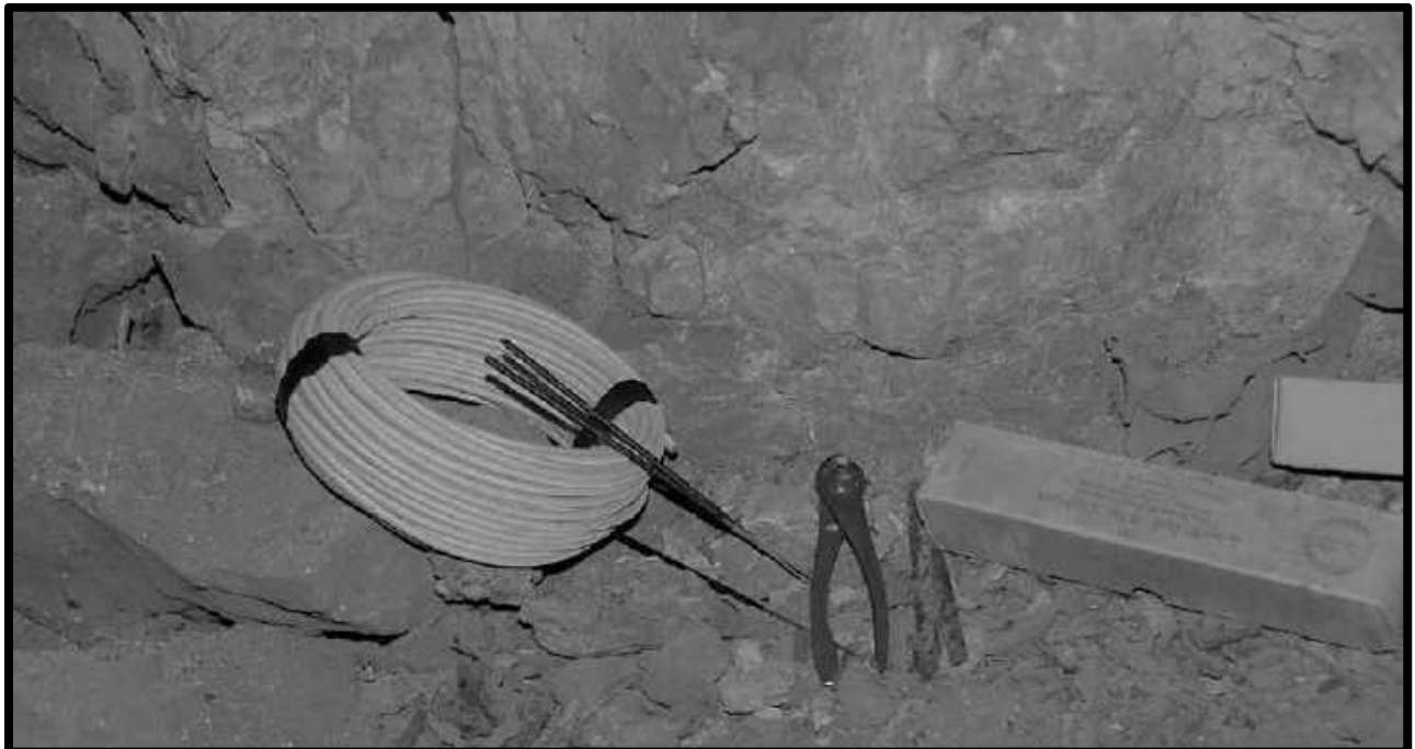
FUSE (FIRE) WITH SPITTERS AND CAP CRIMPERS 3 RD LEVEL, SOUTHWEST MINE, 61 CROSSCUT
