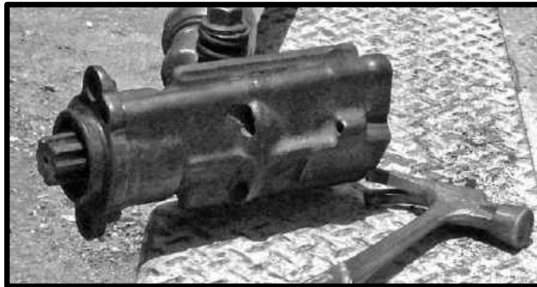
CYLINDER (DEF. 1) FOR A GARDNER- DENVER S63F JACKLEG
