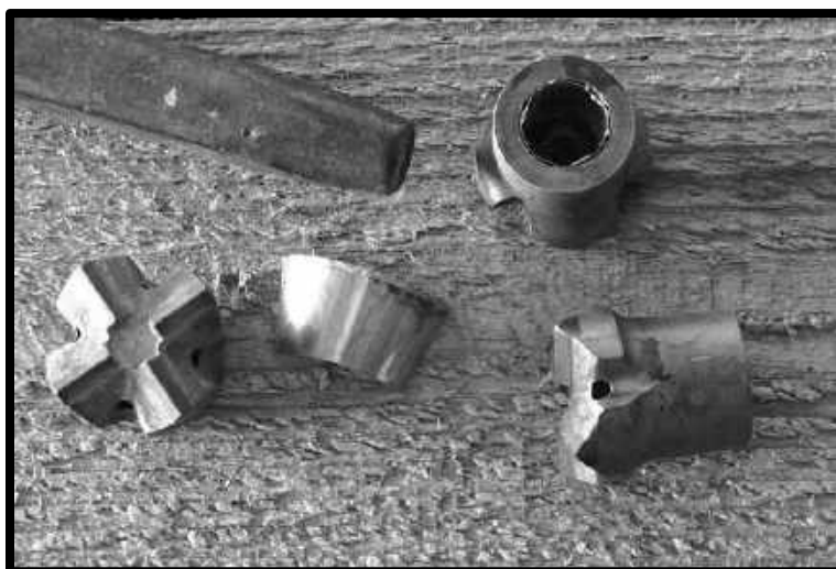
KNOCK OFF DRILL BITS SHOWING THE END OF THE DRILL STEEL IN THE UPPER LEFT CORNER AND A BRASS SHIM IN THE CENTER
