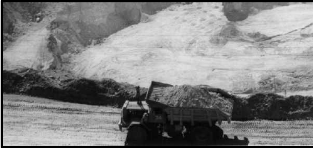
BERM ALONG A HAUL ROAD IN THE LAVENDER PIT
