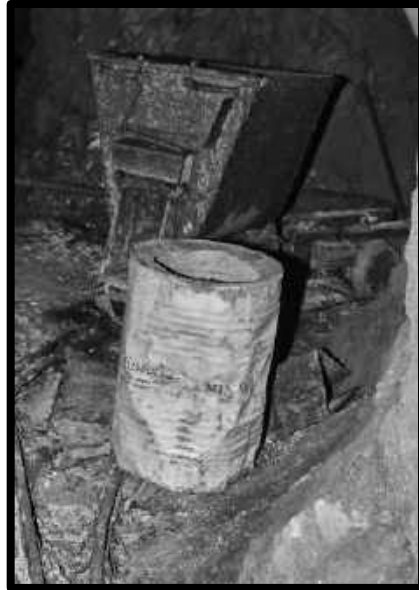
CARBIDE CAN A 100 LB. CARBOLITE BRAND WITH AN ABANDONED QUEEN ROCKER AND TIMBER TRUCK IN THE BACKGROUND AT THE INTERSECTION OF 10 AND 9 CROSSCUTS 6 TH LEVEL SOUTHWEST MINE
