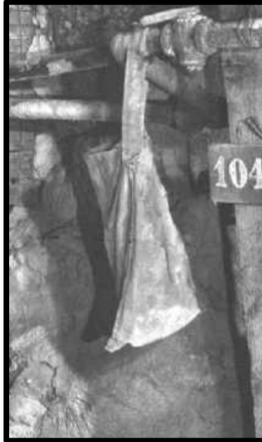
POWDER SACK HANGING FROM A WATER LINE ON THE 1500 LEVEL JUNCTION MINE IN 104 CROSSCUT.
