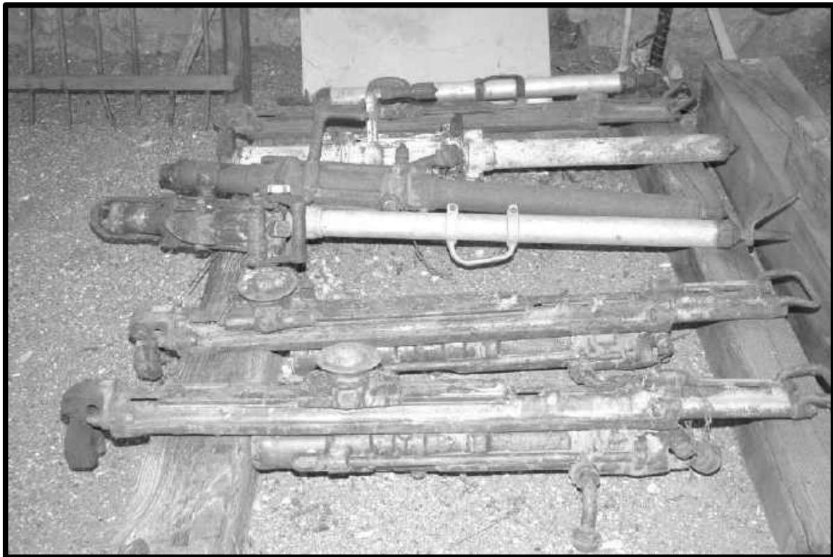
MACHINES , FROM FRONT TO BACK TWO GARDNER-DENVER CF 89 DRIFTERS, THOR 390 JACKLEG, TWO INGERSOLL-RAND 45 STOPERS (ONE SLIGHTLY MODIFIED) A GARDNER-DENVER CF 89 AND A LEG FOR A JACKLEG.
