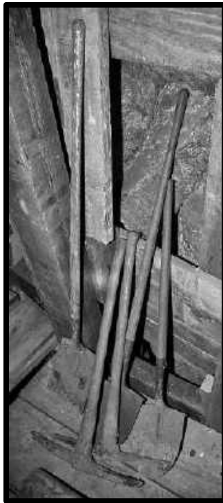
MUCK STICK(S) BEHIND TWO PICKS AT THE COPPER QUEEN INCLINE, 3 RD SW. STATION.
