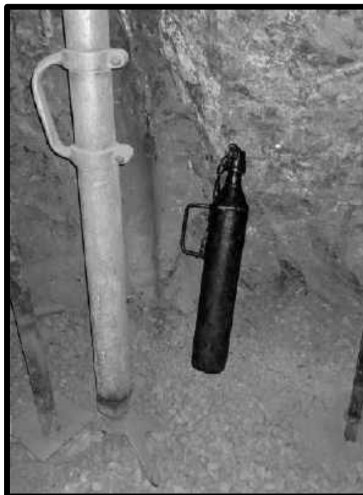
OIL BOTTLE NEXT TO AN AIR LEG AT THE QUEEN MINE TOUR
