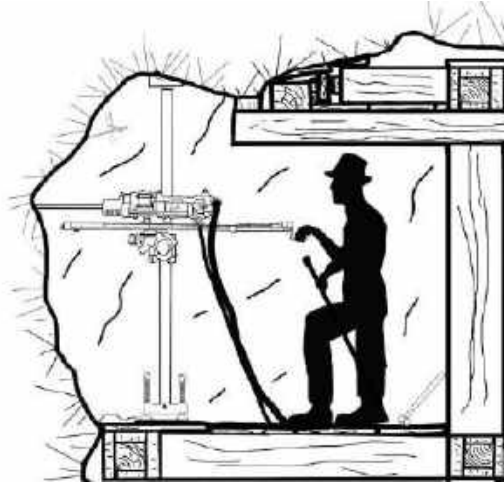
COLUMN WITH DRILL MOUNTED
