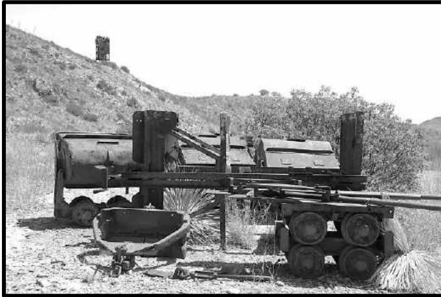
HURRICANE DECK BEHIND A SLUSHER BUCKET AND A STACK OF TIMBER TRUCKS AT THE SHATTUCK MINE.
