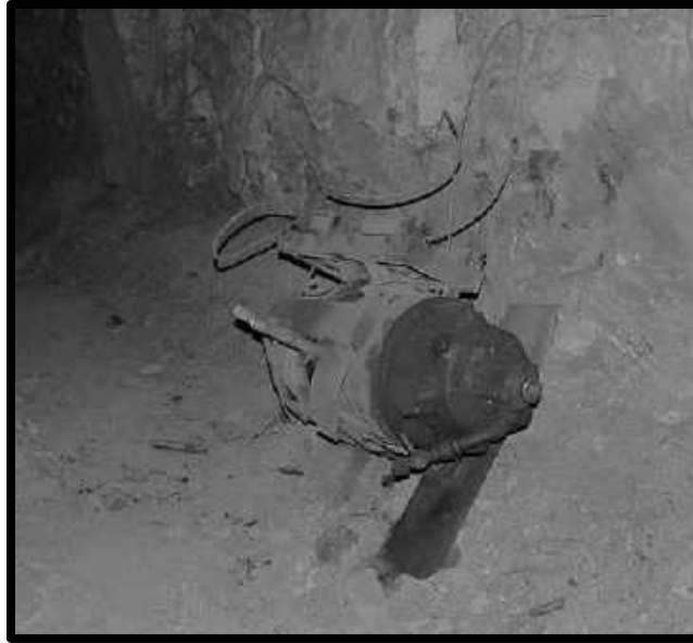
SLUSHER ON SKIDS 61 CROSSCUT, 3 RD LEVEL, SOUTHWEST MINE
