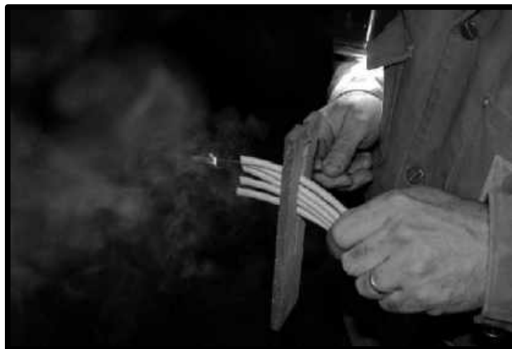
SPITTER BOARD WITH FUSES BEING SPIT.
