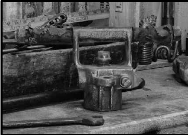
BACKHEAD FOR A COCHISE TYPE 36 PLUGGER REMOVED FROM A DRILL
