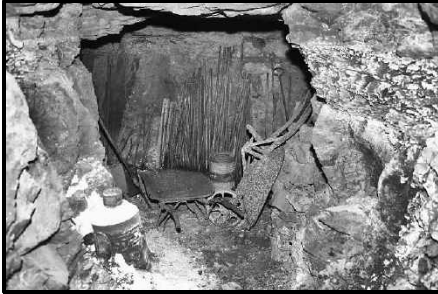
STEEL LEANING AGAINST THE RIB(WALL) OF AN ABANDONED TOOL ROOM ON THE 6 TH LEVEL SOUTHWEST MINE.
