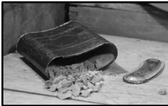
CARBIDE FLASK POCKET STYLE WITH CARBIDE (CALCIUM CARBIDE) SPILLING OUT.
