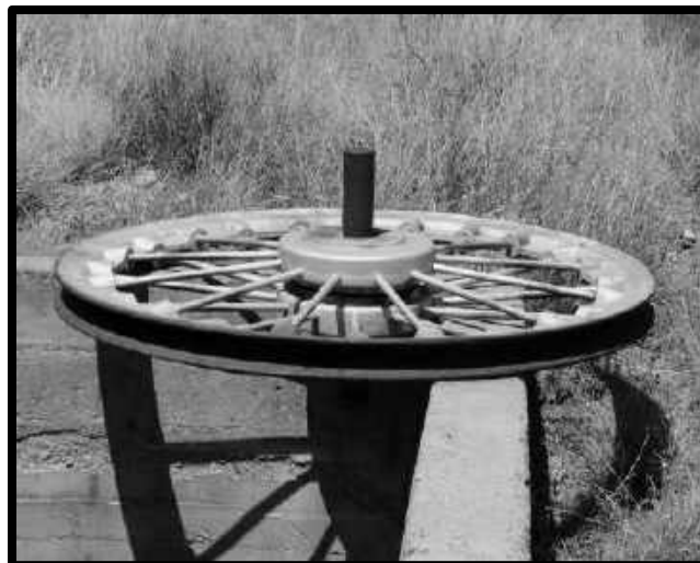
SHEAVE WHEEL , A SPARE STORED AT THE SHATTUCK MINE.
