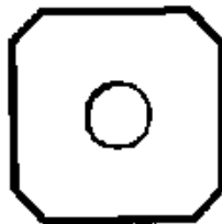
QUARTER OCTAGON DRILL STEEL IN CROSS SECTION CROSS
