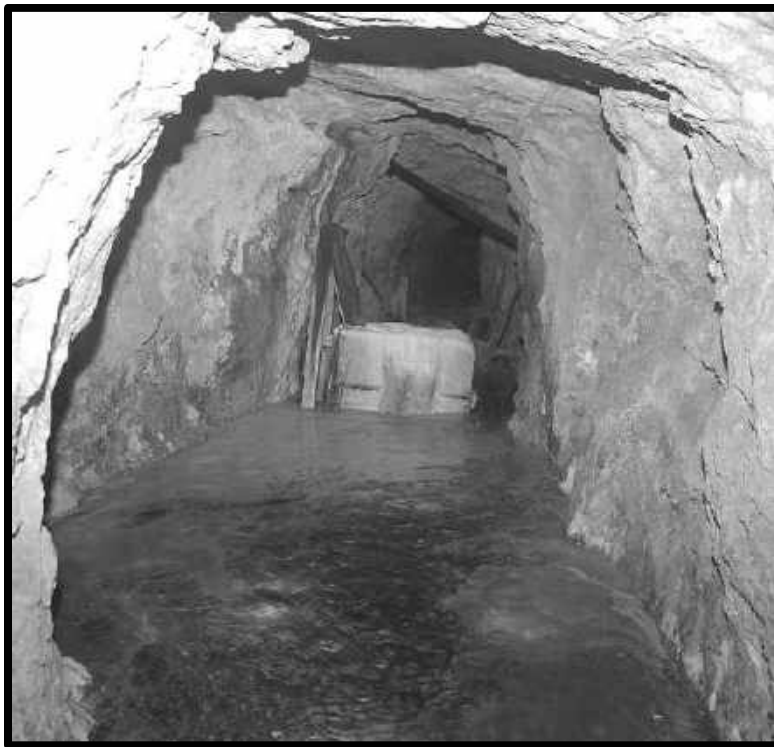
MINE WATER ABOUT 18 INCHES DEEP WITH A MINE CAR TUB RESTING IN IT. HIGGINS TUNNEL
