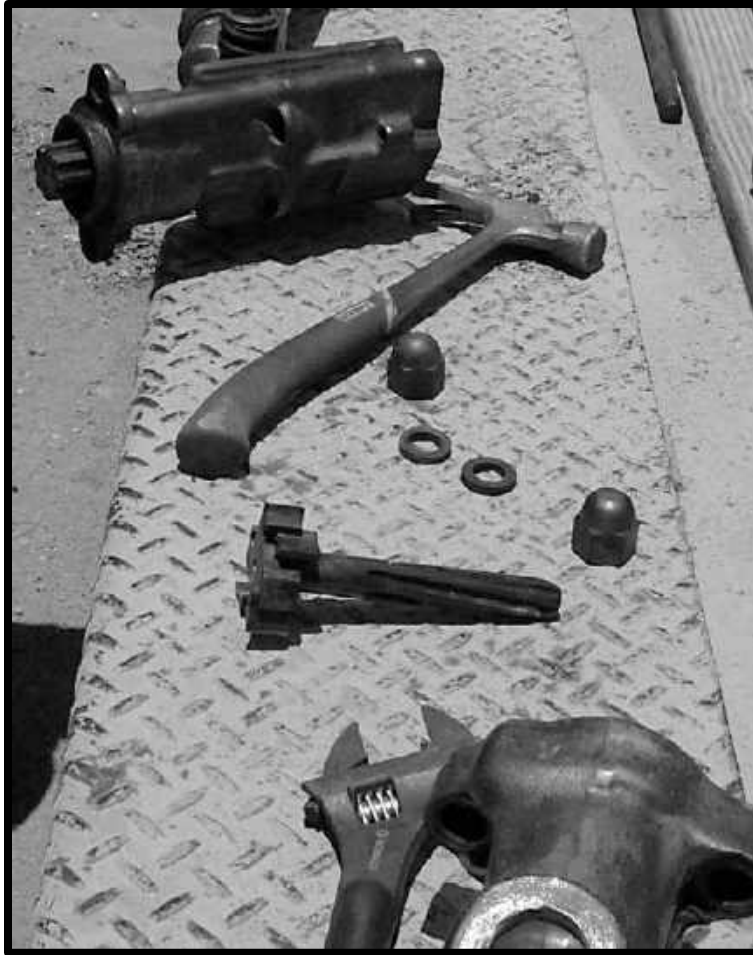
RIFLE BAR FOR A GARDNER-DENVER S63F JACKLEG REMOVE DURING REPAIRS AT THE QUEEN MINE TOUR
