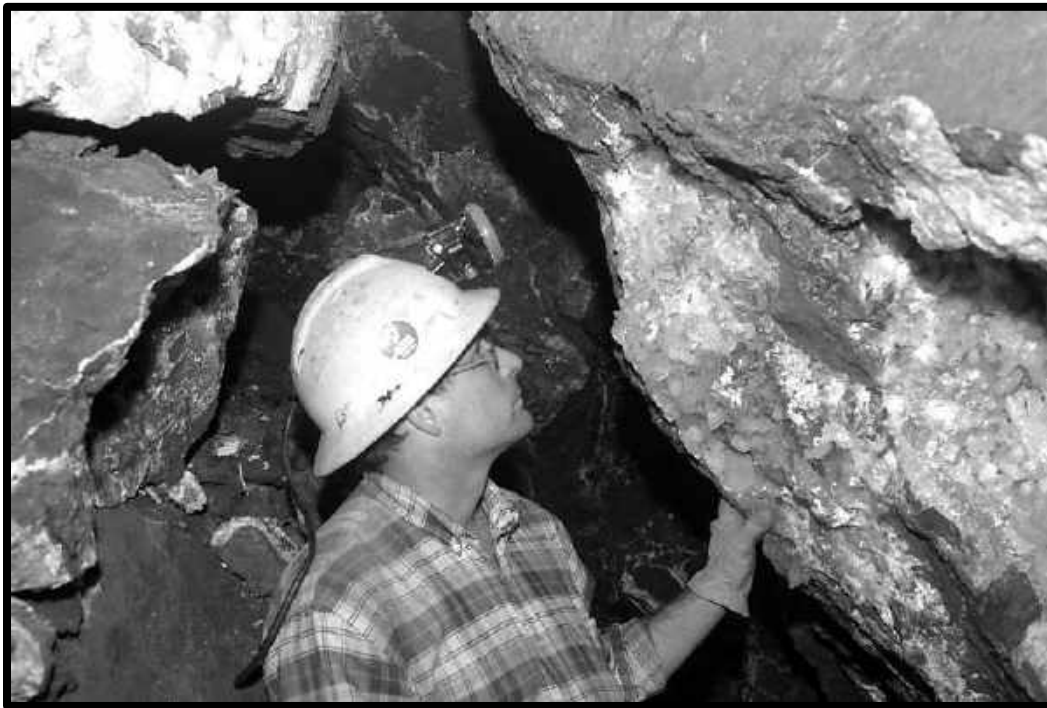
VUGGY GROUND BALLPARK STOPE 7 TH LEVEL SOUTHWEST MINE
