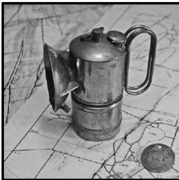
SUPERINTENDENT'S LAMP DEWAR MODEL 16, RESTING ON A SHATTUCK MINE MAP WITH A MAN TAG.
