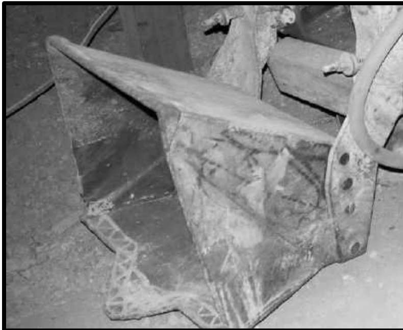
HARDFACING ON A TRIANGULAR PATTERN ON A MUCKING MACHINE BUCKET.
