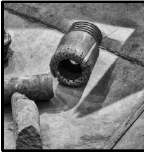
BIT FOR A DIAMOND DRILL WITH PIECES OF CORE.
