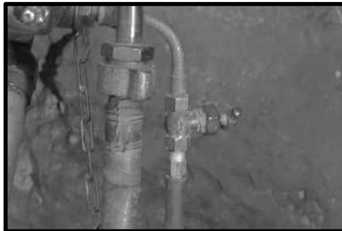
GOOSENECK ATTACHED TO A GARDNER-DENVER S63F JACKLEG
