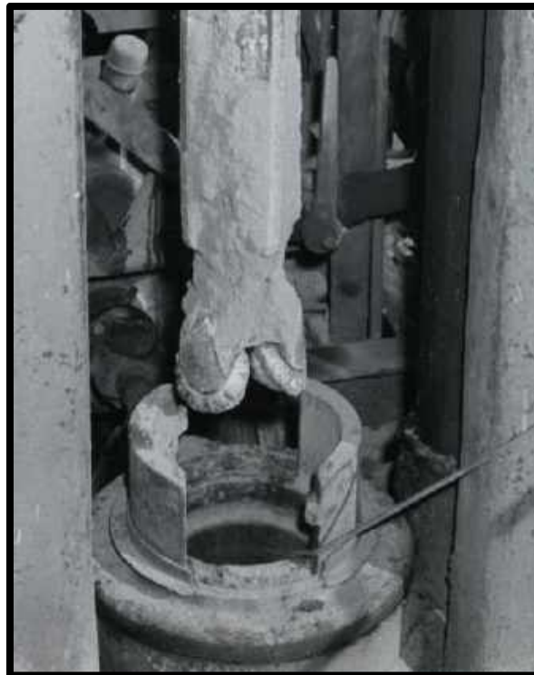
TRICONE BIT ON A DRILL RIG IN THE LAVENDER PIT.
