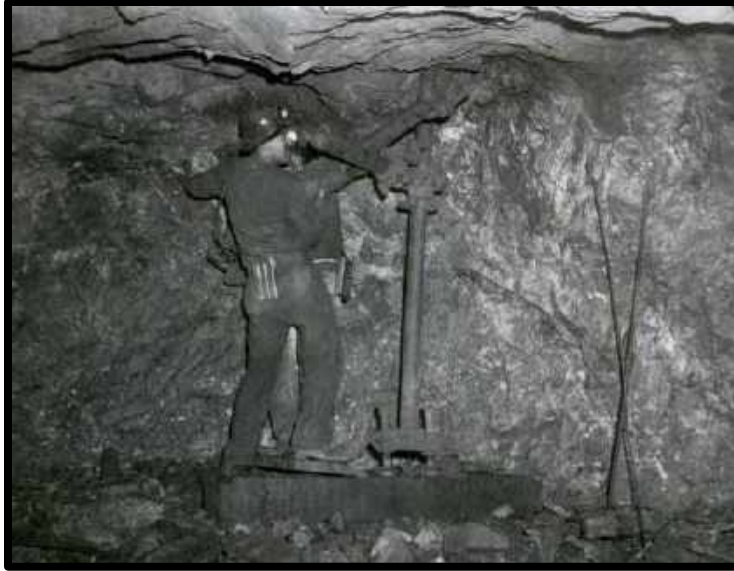
SETUP OF A CF 89 DRIFTER ON A BAR AND COLUMN C-1952
