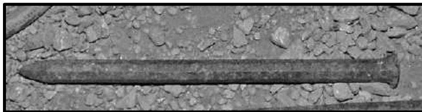
MOIL ON 3 RD LEVEL OF THE SOUTHWEST MINE.
