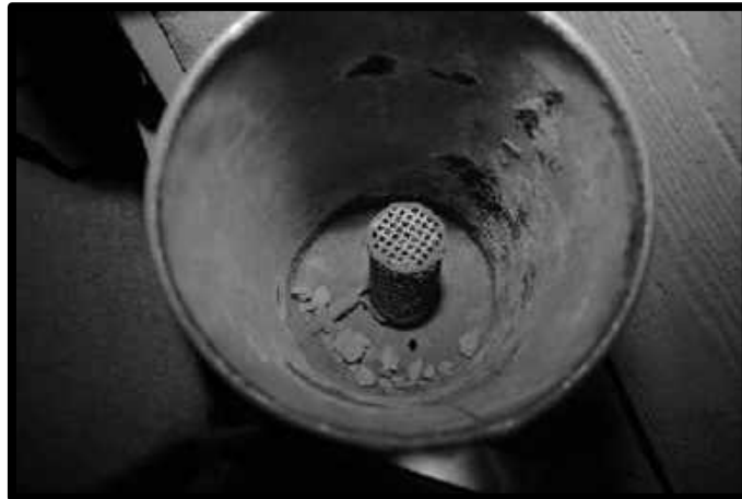
SPITTER CAN (RIGHT) AND THE SAME CAN(BELOW) OPEN TO SHOW THE WIRE MESH COVERING THE LIGHT BULB
