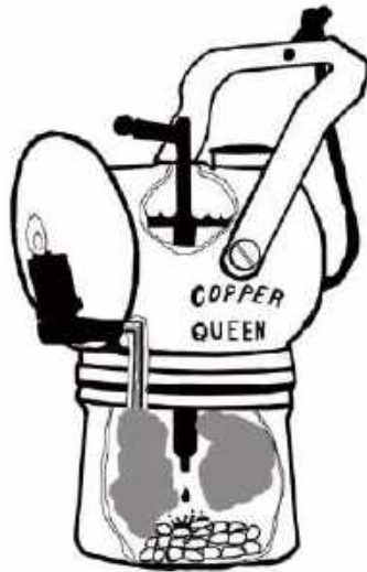
CARBIDE LAMP, CUTAWAY SHOWING WATER AND CARBIDE CHAMBERS.
