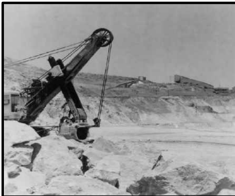
STICKS ON A SHOVEL IN THE LAVENDER PIT WITH THE CONCENTRATOR IN THE BACKGROUND.
