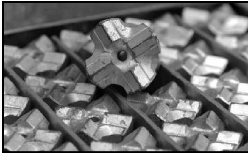
CARBIDE BIT , A BRAND-NEW BIT SITTING ON A BOX OF NEW BITS.
