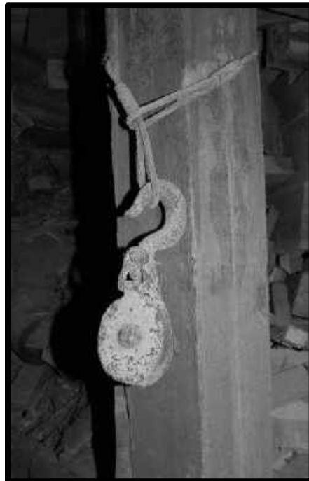
SLUSHER BLOCK HANGING FROM A SLING IN 61 CROSSCUT, 3 RD LEVEL, SOUTHWEST MINE.
