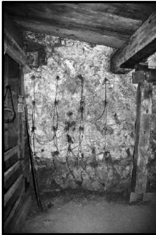
BURN CUT DEMONSTRATION BLASTING ROUND AT THE QUEEN MINE TOUR
