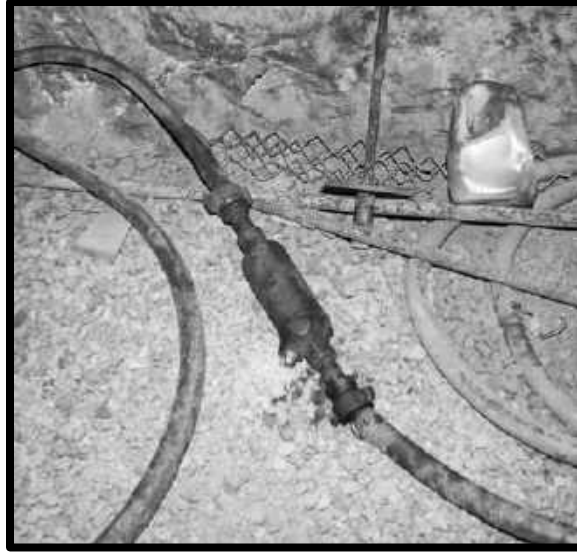
OILER (DEF.2) HOOKED UP IN LINE WITH A DRILL.
