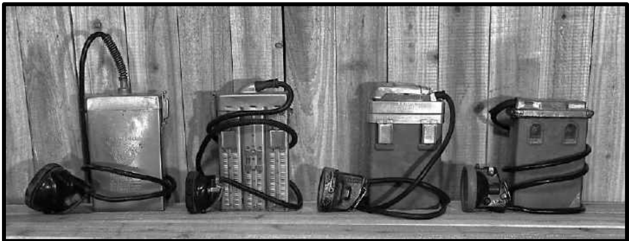
LAMP(S) THE TYPES OF ELECTRIC LAMPS USED BY MINERS IN BISBEE. FROM LEFT TO RIGHT EDISON MODEL K, EDISON MODEL P, EDISON R4 AND WHEAT MARK II
