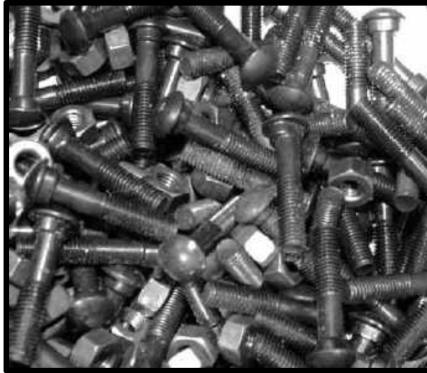
TRACK BOLT(S) IN A STEEL KEG SOUTHWEST MINE 3 RD LEVEL 30 CROSSCUT.
