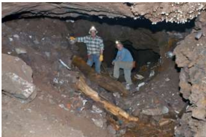
Figure 1.7.15: Two of the authors in the crosscut that intercepted this cave. The whole of entire ceiling is the top of the oxidation cave, as shown by the scattered calcite speleothems. The left portion of the cave was completely backfilled while the right portion was largely open. Note the goethite and hematite wall on the right.
