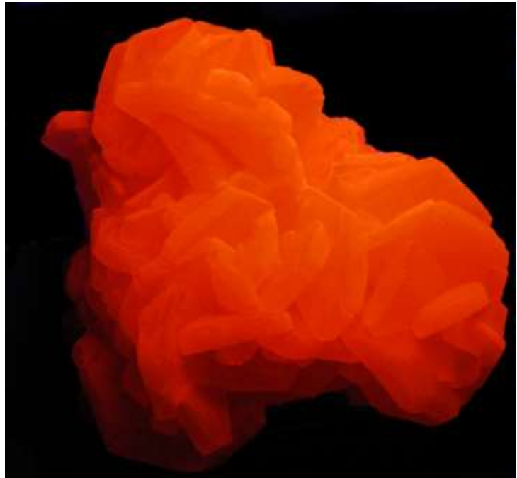
Figure 2.6.6: Hydrothermal calcite response to shortwave UV light, 2566 level Campbell Mine, specimen - 6.2 centimeters.
