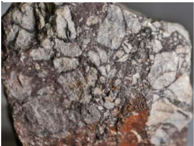
Figure 2.6.9: "Silica Breccia" composed of siliceous, altered limestone with silica fragments and minor goethite in a groundmass of quartz and specular hematite, Uncle Sam Mine, specimen - nine centimeters.
