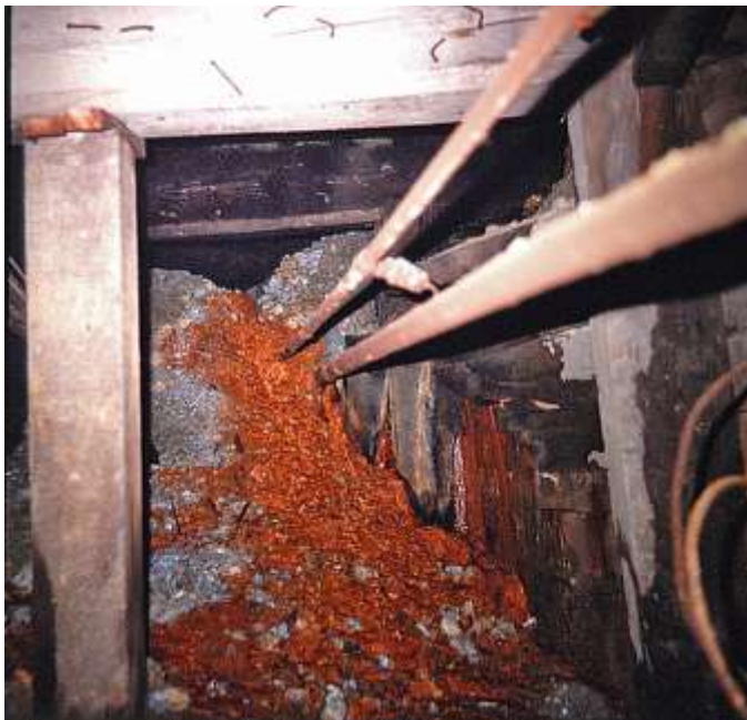
Figure 2.3.4: Acidic, iron-rich solutions, generated by the oxidation of pyrite, depositing iron hydroxide minerals on limestone with some goethite being deposited as darker patches, 2700 level, Junction Mine, vertical view 1.80 meters.
