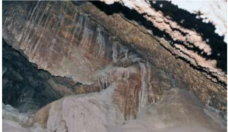
Figure 1.5.14: Sag cave at the intersection with a marginal crack. Note the fine-grained material that has entered the cave from the surface along the marginal crack, 8 th level, Southwest Mine, horizontal view - eight feet.
