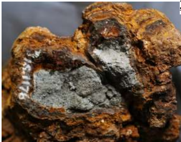
Figure 2.3.2: Goethite formed through the oxidation of pyrite with unoxidized pyrite core, Neptune Mine, Tunnel level, view - 5.5 centimeters, Harvard Mineral Museum collection.
