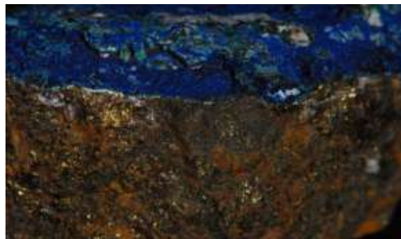
Figure 2.3.3: Azurite veneer developed on oxidizing chalcopyrite, pyrite and bornite. Note the goethite derived from pyrite oxidation, as well as the iron contained in the copper bearing minerals, Gardner Mine, specimen - six centimeters.
