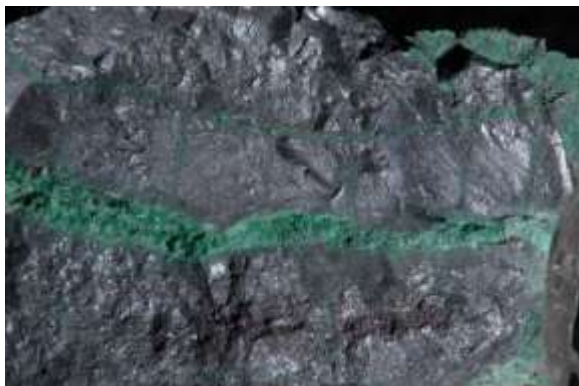
Figure 2.3.12: Chalcocite altering directly to malachite along fractures. Note the openness of the malachite in the center of the specimen, Shattuck Mine, view - 7.7 centimeters.
