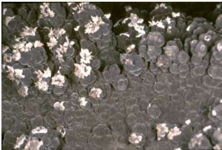
Figure 1.4.12: Brown-black mottramite with minor calcite, 8 stope, 600 level, Shattuck Mine, view – seven inches.
