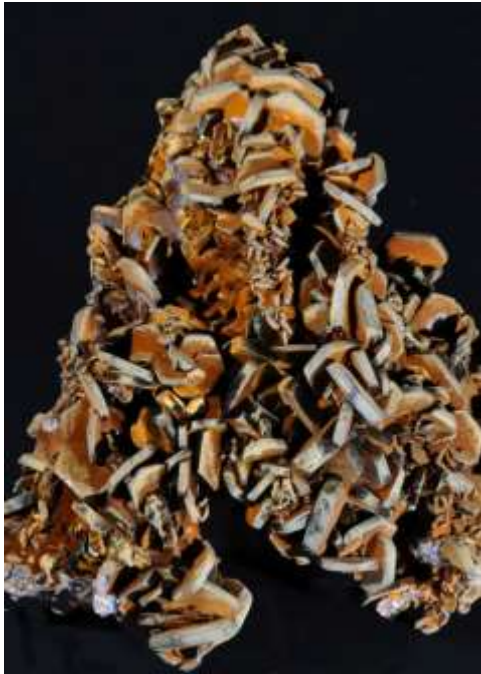
Figure 2.6.5: Pseudo-hexagonal calcite crystals lightly coated with goethite, 2566 level, Campbell Mine, specimen - 17 centimeters.
